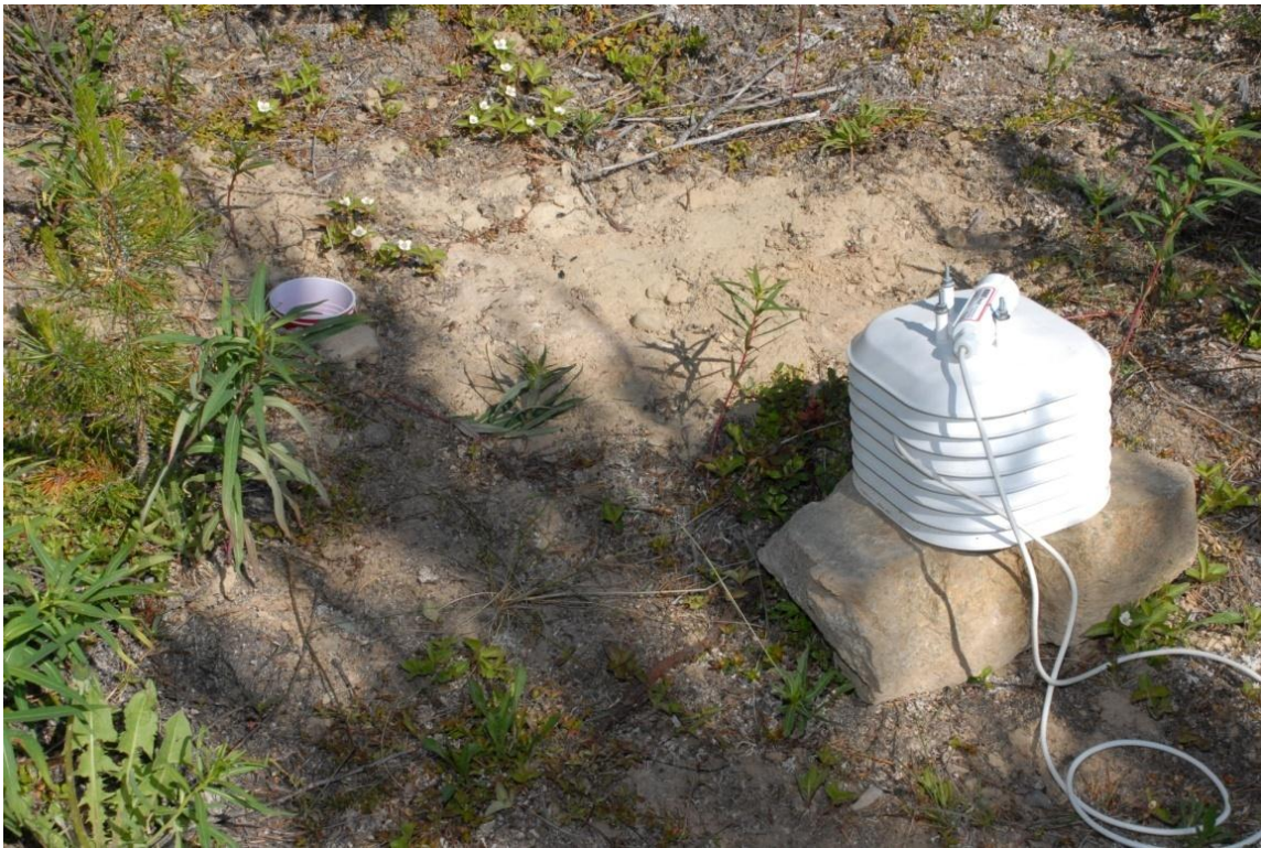
Figure 3. Control site set-up within the Whitehorse Municipal Landfill, with independent pitfall trap and data-logger.
