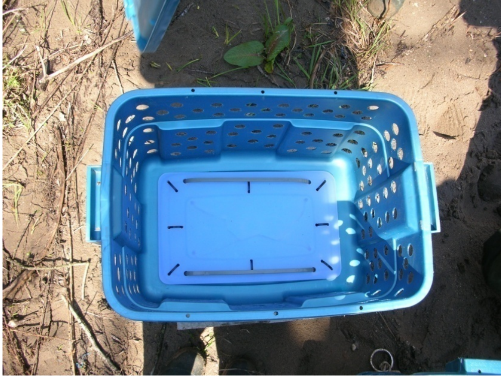
Figure 7.2: Cage modification 2 depicting reinforced bottom with plastic plating and increased number of holes around the exterior.
