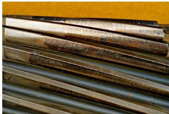
Figure 5.4: Severe Scuffing on the High Speed Pinion [15]
