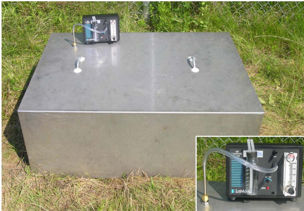
Figure 2.5: Stainless steel sampling hood and outdoor VOCs sampling set-up. Inset: connection of TD sampling tube and pump.
