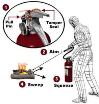
Figure 3.1: The P.A.S.S technique employed to safely extinguish a fire is an important aspect of fire safety. Image taken from United States Department of Labor [86].
