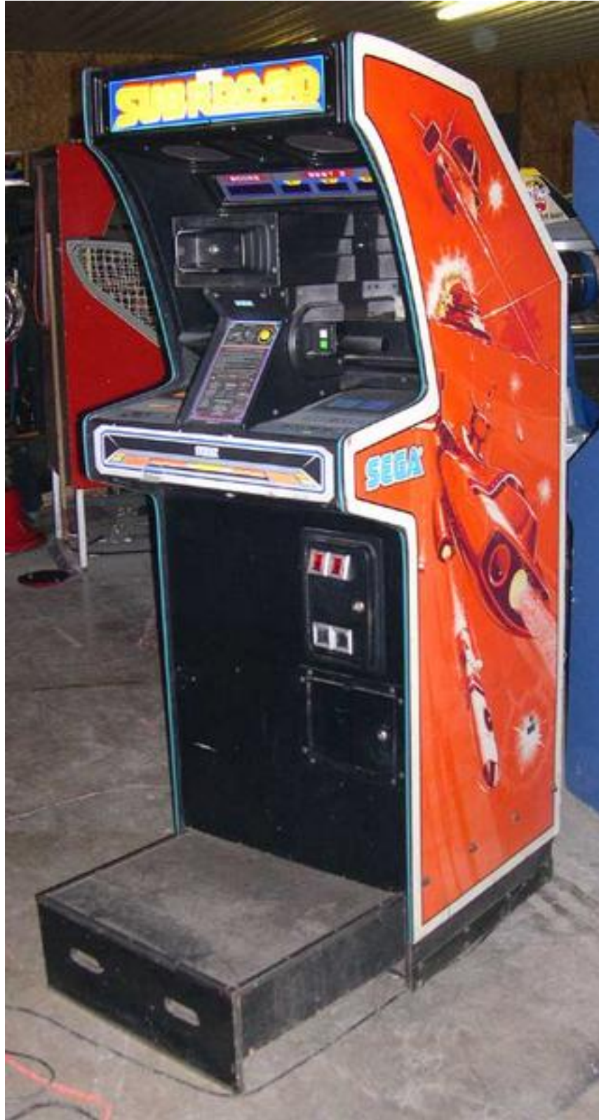
Figure 2.14: SubRoc-3D is an arcade game released in 1982 by Sega, and the first such game to provide a three-dimensional image to the player. It employed a display that delivers individual images to each eye, achieved by using a viewer with spinning discs to alternate left and right images to the player's eye from a single monitor [115].
