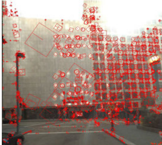
Figure 3.3: SIFT features extracted from a cropped reference image using s_l = 3 , s_c = 0.04 , s_e = 10 and s_\sigma = 0.9 . We use these parameter values for extracting SIFT features from our geo-tagged reference dataset. For the image shown here a total of 2336 SIFT features were extracted.
