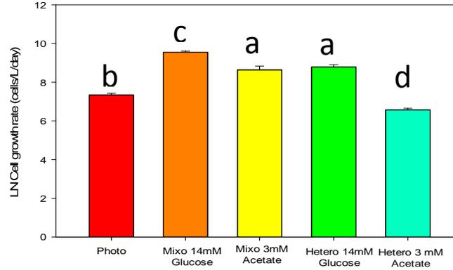
Figure 20: *Chlorella* 04 Corbett Creek tested under the three conditions photoautotrophic, mixotrophic, and heterotrophic growth. Significant differences are denoted by different letters. Data was ln transformed to ensure normal distribution. Samples were run in triplicate under each condition simultaneously in the algaetron growth chamber.
