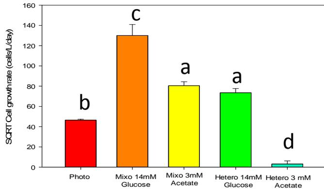
Figure 19: *Chlorella* 03 Corbett Creek tested under the three conditions photoautotrophic, mixotrophic, and heterotrophic growth. Significant differences are denoted by different letters. Data was transformed by taking the square root of the raw data to ensure normal distribution. Samples were run in triplicate under each condition simultaneously in the algaetron growth chamber.
