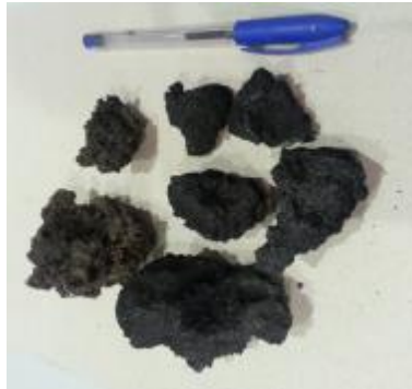
Figure 3.12 Agglomeration occurred in the bubbling fluidized bed.
