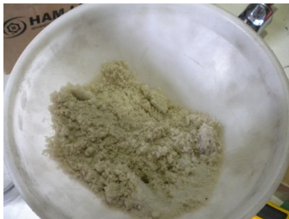
Figure 3.10 Moist silica sand if dampens before the experiments.
