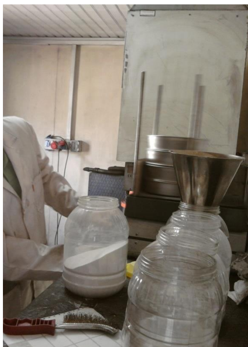
Figure 3.2 Sieving silica sand into desired particle size
