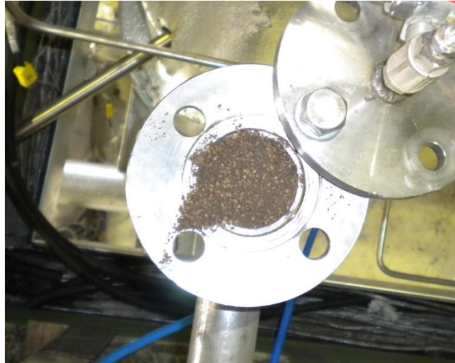
Figure 3.9 Coal samples stuck in screw-feeder.
