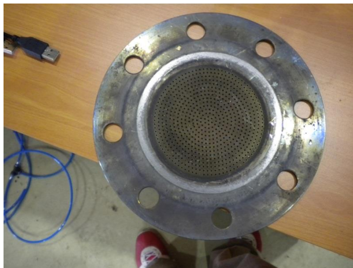
Figure 3.7 External view of the distributor plate when dismantled.
