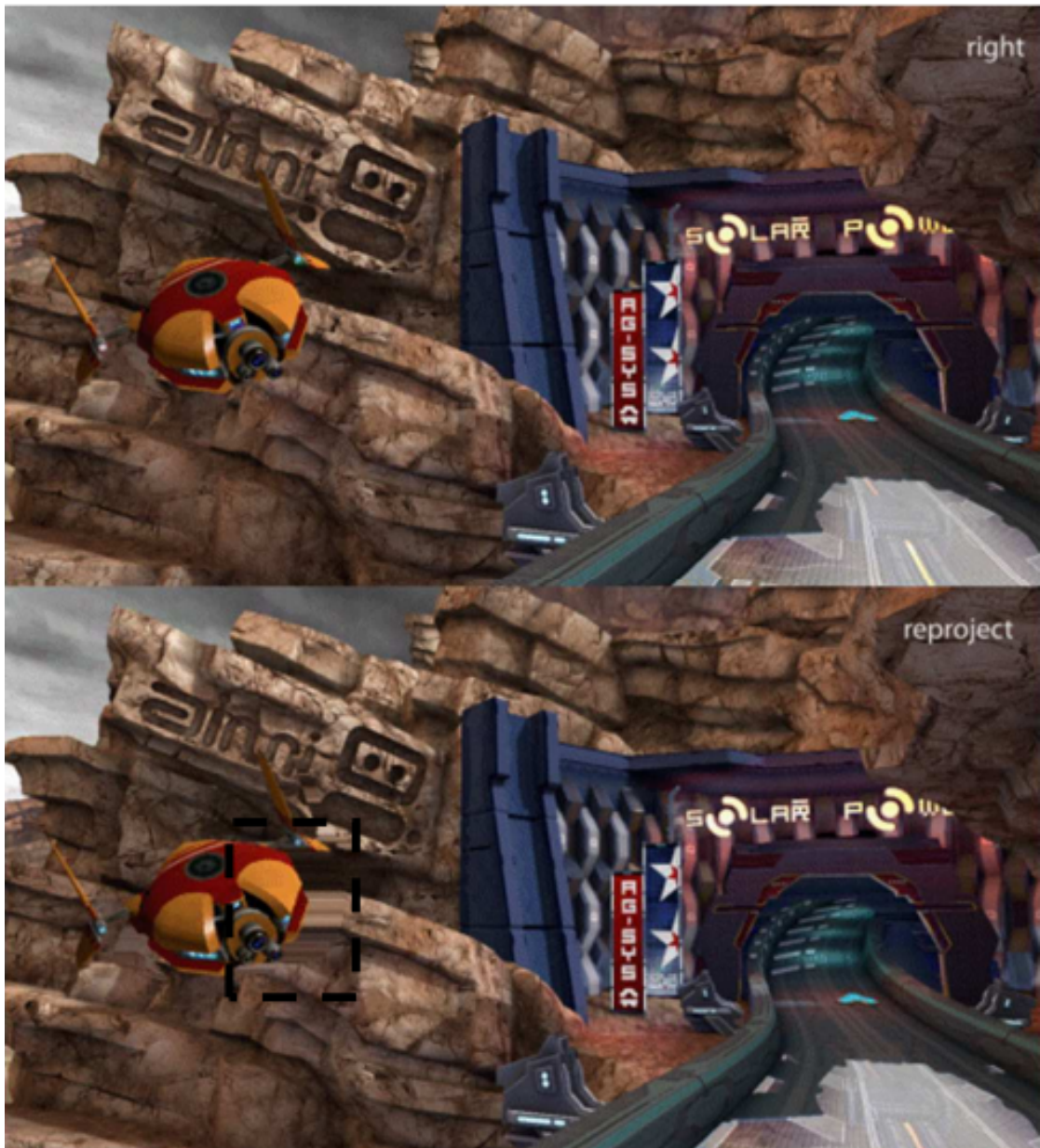
Figure 2.11: Image depicting the creation of a hole when creating the image of the second eye from the depth buffer, using the reprojection technique [19]. Copyright Sony 2013.
