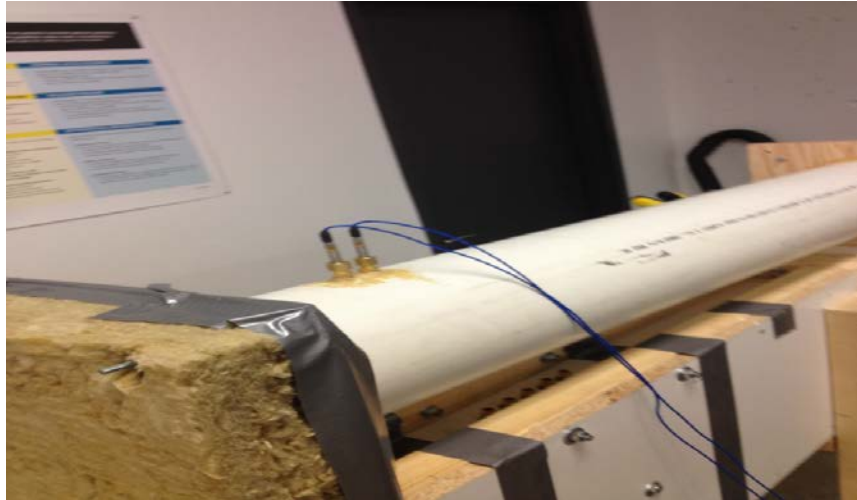
Figure D.3: Impedance tube with the two microphones inserted along with the 3 inch acoustical material installed and well sealed.
