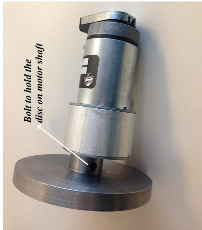
Figure 2.14: Momentum disc attached with motor
