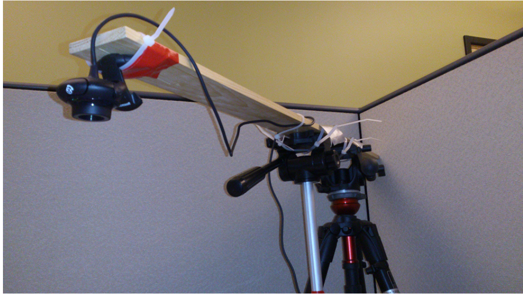
Figure 5.5: The camera rig used to help PlayTIME track AR markers (labelled as (3) in Figure 5.2). The camera was suspended approximately 60cm above the centre of the workspace using a wood plank attached to a pair of tripods.
