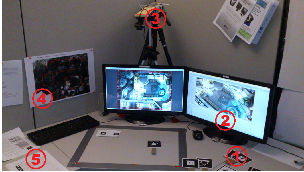
Figure 5.2: An overview of the study setup showing the different components. Pictured here are five different components of the setup: (1) the workspace complete with AR paddles; (2) the dual-monitor setup used to display the activity systems; (3) the setup used to hold the camera in place; (4) a map of the scenario to be worked on; and (5) the notes that were provided to the participants (observer section not pictured).
