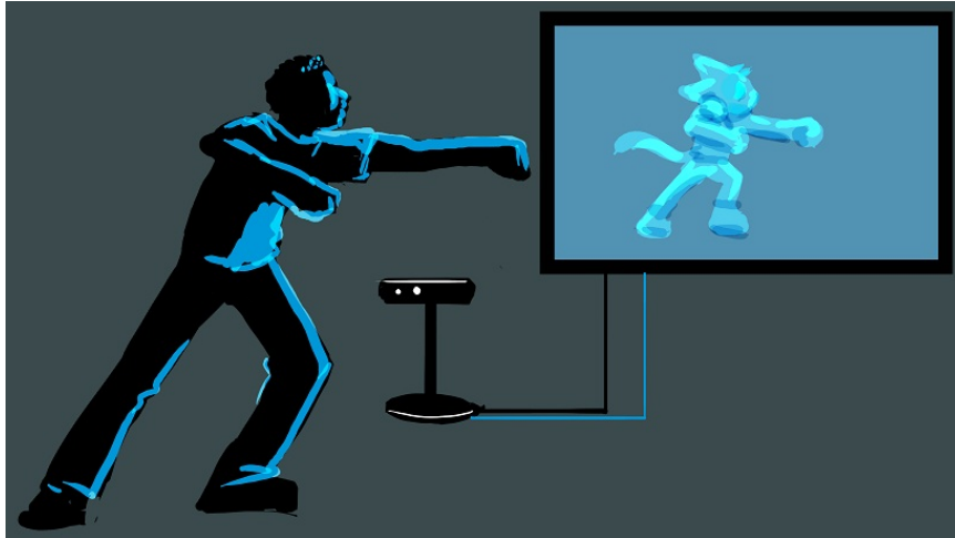
Figure 4.11: A Kinect is used to capture full-body gestures to create animation sequences.
