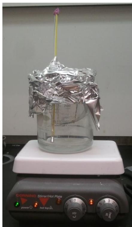
Figure 3-4: Schematic (top) and Photo (bottom) of an Acetone Vapour Bath in a Double Boiler System
