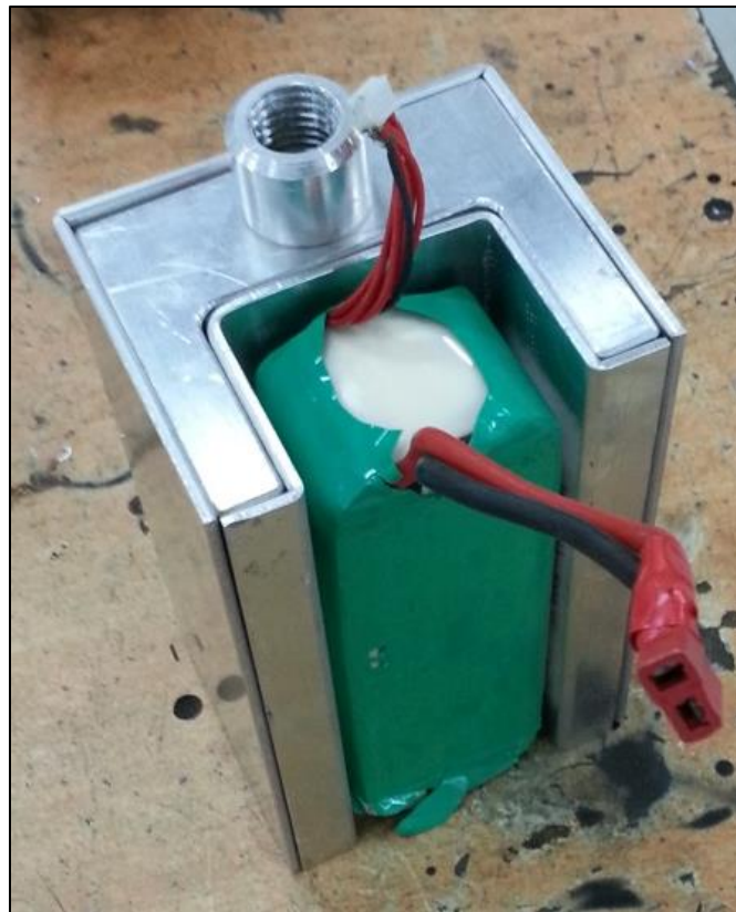
Figure 5.4 Dry fit setup of the battery and the PCM jacket
