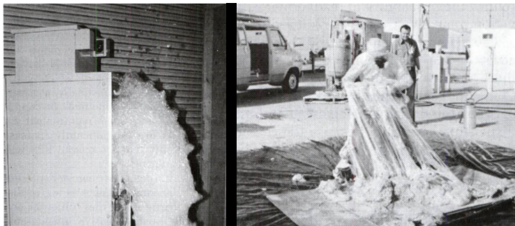
Figure 3.7: Example dispensable barriers, L: aqueous foam, R: adhesive foam [5].
