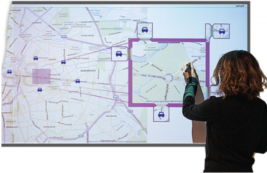
Fig. 2.3 Screenshot image of the © Canyon information visualization technique by Ion et al. [89]. This technique attaches a small inset to the detailed view when an object moves beyond its boundaries.
