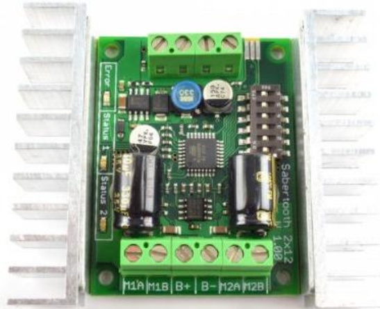
Figure 4.16. Sabertooth dual 12A 6V-24V regenerative motor driver
