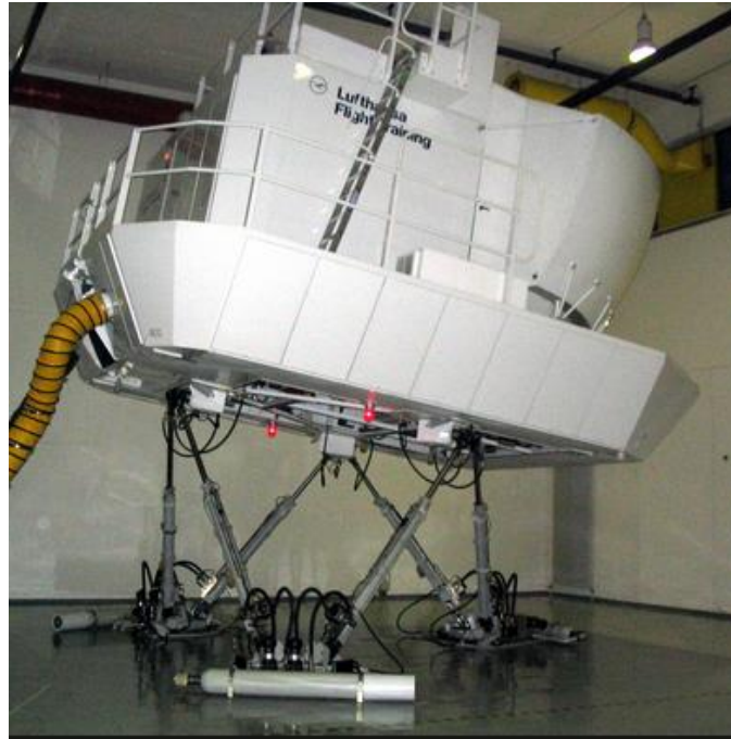
Figure 2.1. Parallel mechanism used in flight simulator [61]
