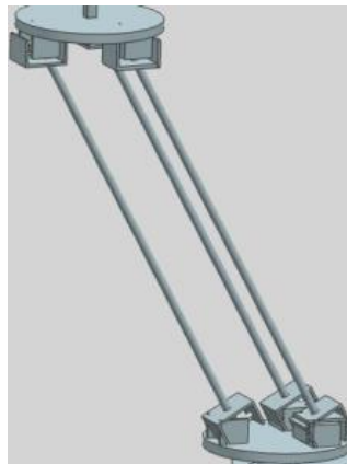
Figure 3.2. Pure-translational universal joint
