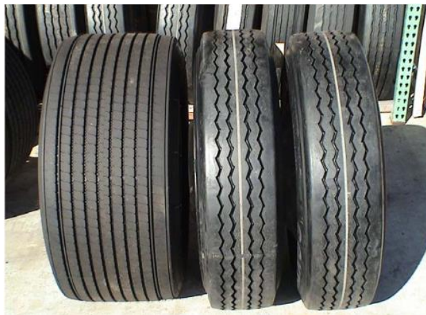
Figure 1-3 Wide-base tire vs dual tire [5]
