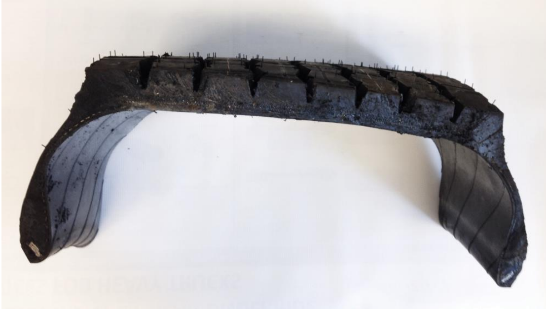
Figure 2-5 Physical Michelin XOne Line Energy T tire Section cut
