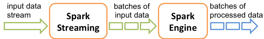
Figure 2.2: Spark Streaming General Processing Flow
