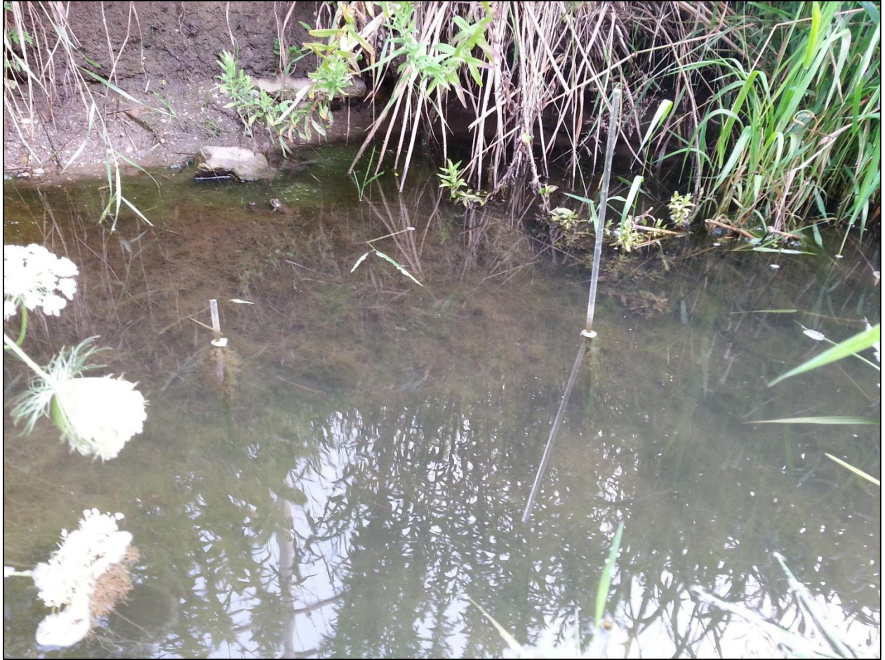
Figure 3.2: Representative picture of algal assay acrylic rod placement. Rod length was dependant on water depth.
