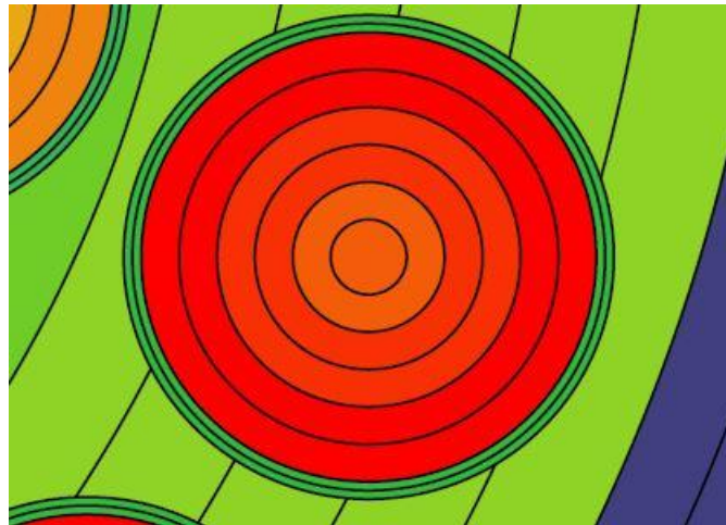
Figure 5.3 Fine spatial discretization at fuel pin level in the lattice cell model.
