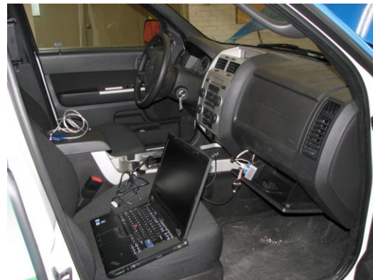
b) The data logger installation beneath passenger seat
