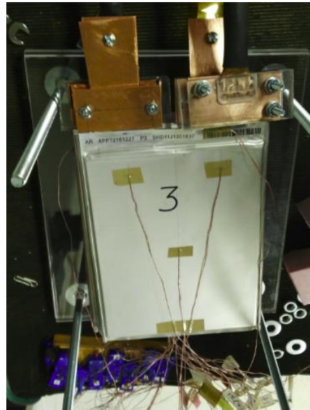
b) Picture of actual cell with thermocouple
