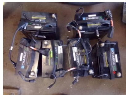
b) First six modules connected in series
