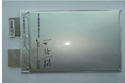
Figure 3.1: 20Ah LiFePO 4 lithium-ion prismatic cells.
