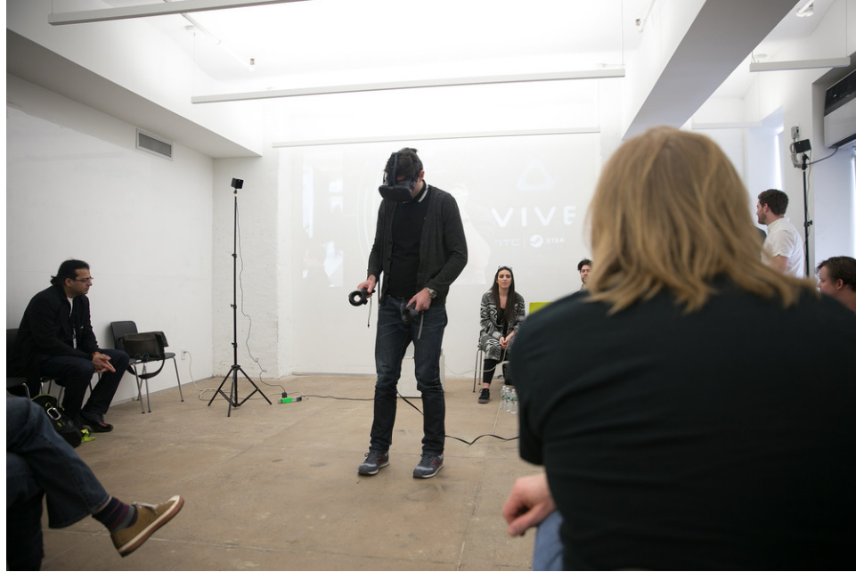
Figure 2.6: A typical room-scale VR setup. The tracking sensors are raised above the user and a large open space is available for free movement [70].
