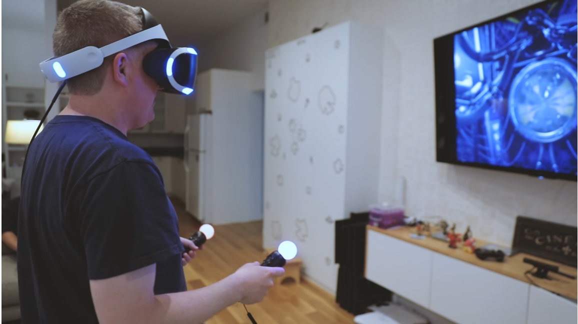
Figure 2.5: A typical standing VR setup. The tracking sensor is directly below the television and the user is standing a moderate distance away [112].
