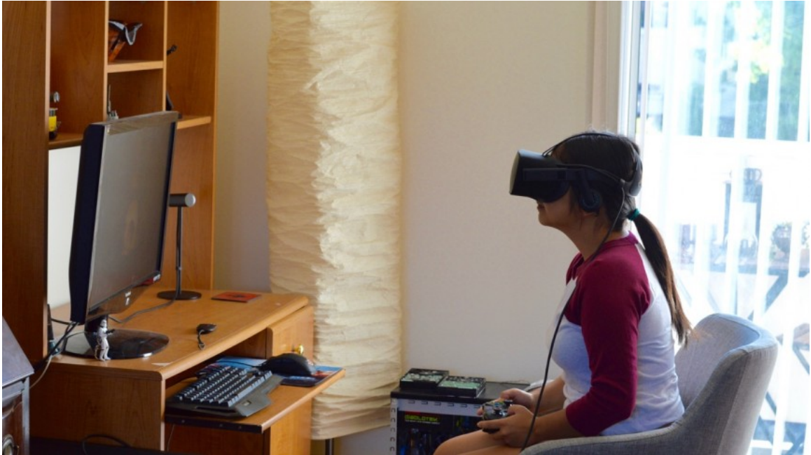
Figure 2.4: A typical seated VR setup. The tracking sensor is on the left beside the monitor and the user remains seated in a chair a short distance away [77].
