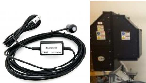
Fig. 3.1 Vernier pyranometer and OAI Trisol TSS-208 Class AAA solar simulator.
