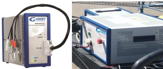
Fig. 3.3 Gamry Instruments Reference 3000 and Reference 30k booster.
