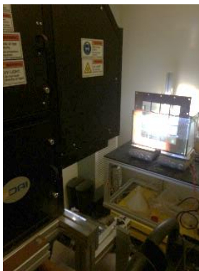
Fig. 3.26 Measurement of photo-responsivity of \text{Cu}_2\text{O} coated cathode plate.
