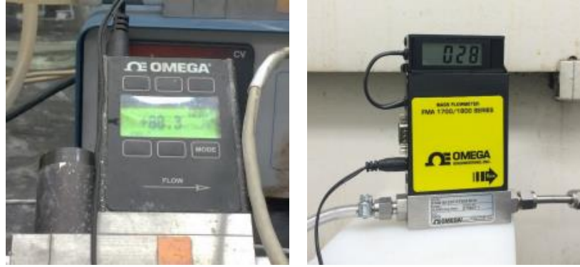
Fig. 3.8 The mass flow meters used in the experiments (OMEGA FMA 1600 and FMA 1800 Series).
