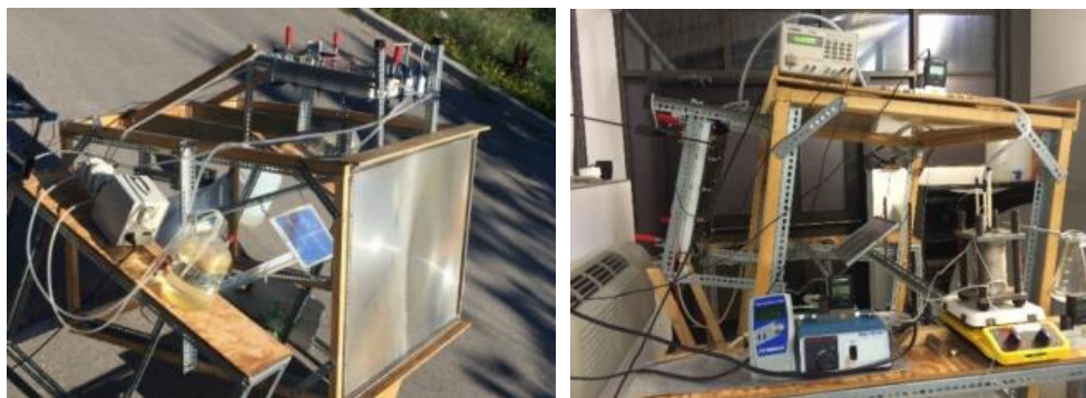
Fig. 3.34 Integrated system for photoelectrochemical hydrogen and ammonia production unit.
