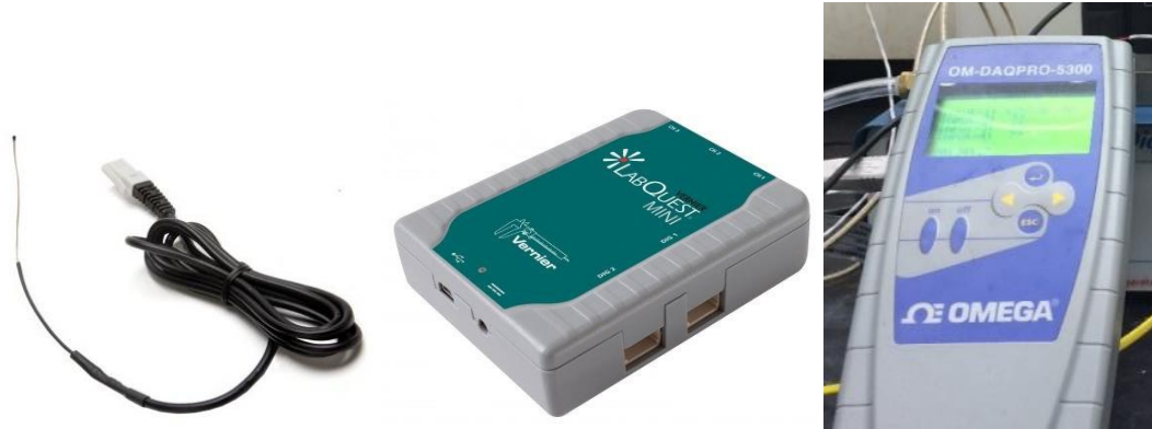
Fig. 3.7 (a) The surface temperature sensor used in PV cell, (b) LAB QUEST data acquisition unit and (c) OM-DAQPRO-5300 temperature logger.
