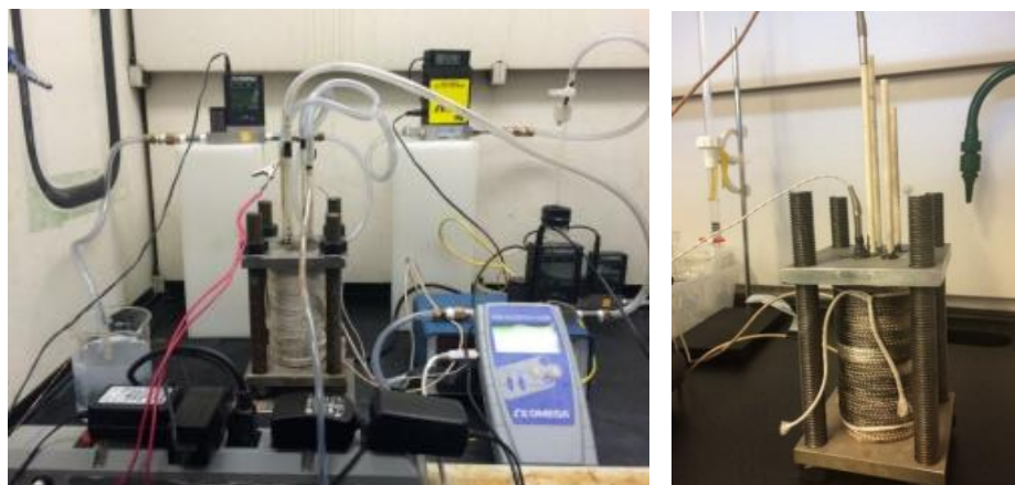
Fig. 3.32 Heating tape used around the alumina crucible and experimental setup with flowmeters, temperature controller and tubing.
