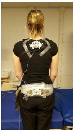
Figure 4.7 Participant wearing vest and belt harnesses securing both rigid bodies and accelerometer-based sensors.
