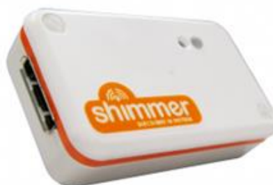
Figure 4.5 Accelerometer-based sensor used during data collection.
