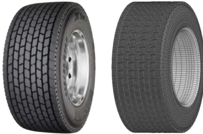
Figure 2-10: Comparison of Reid's Virtual FEA Wide Base Tire (Right) and the Michelin Tire (Left) [27]
