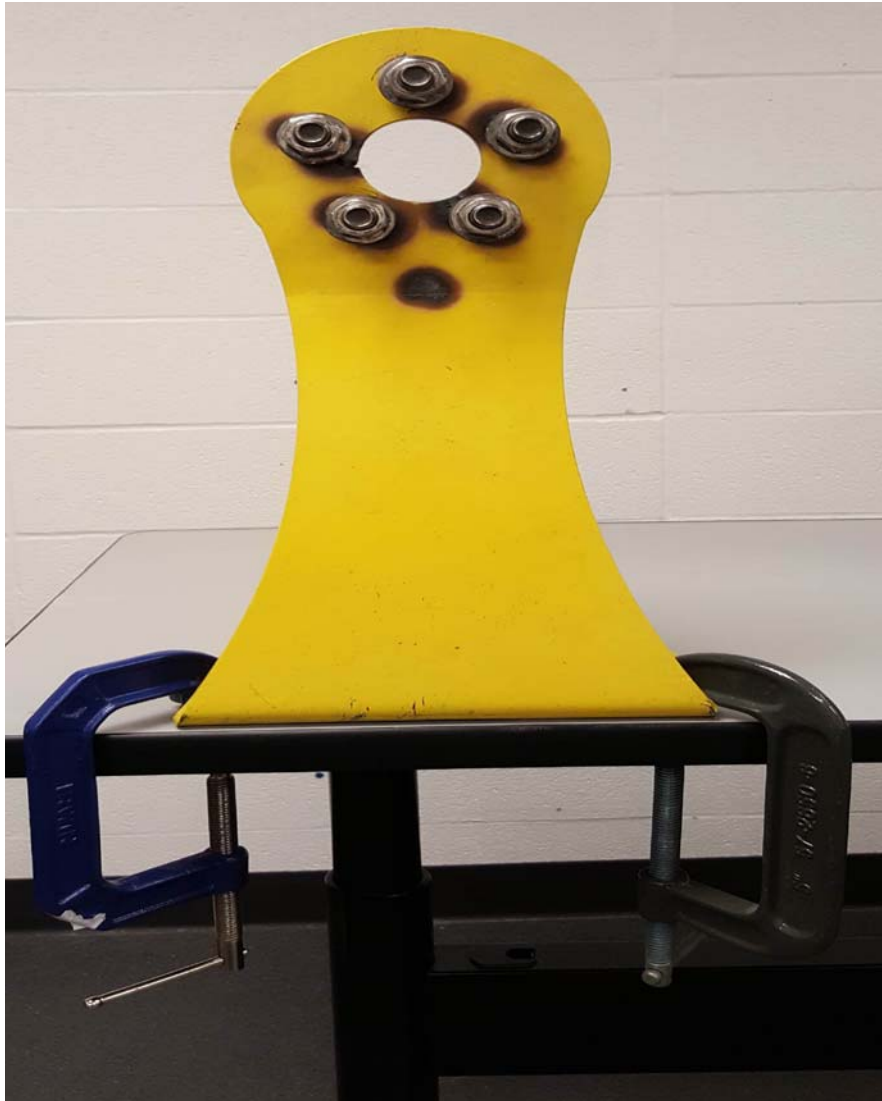
Figure 5: Experimental setup involving a custom steel apparatus designed to emulate the position of lug nut bolts on an automobile.
