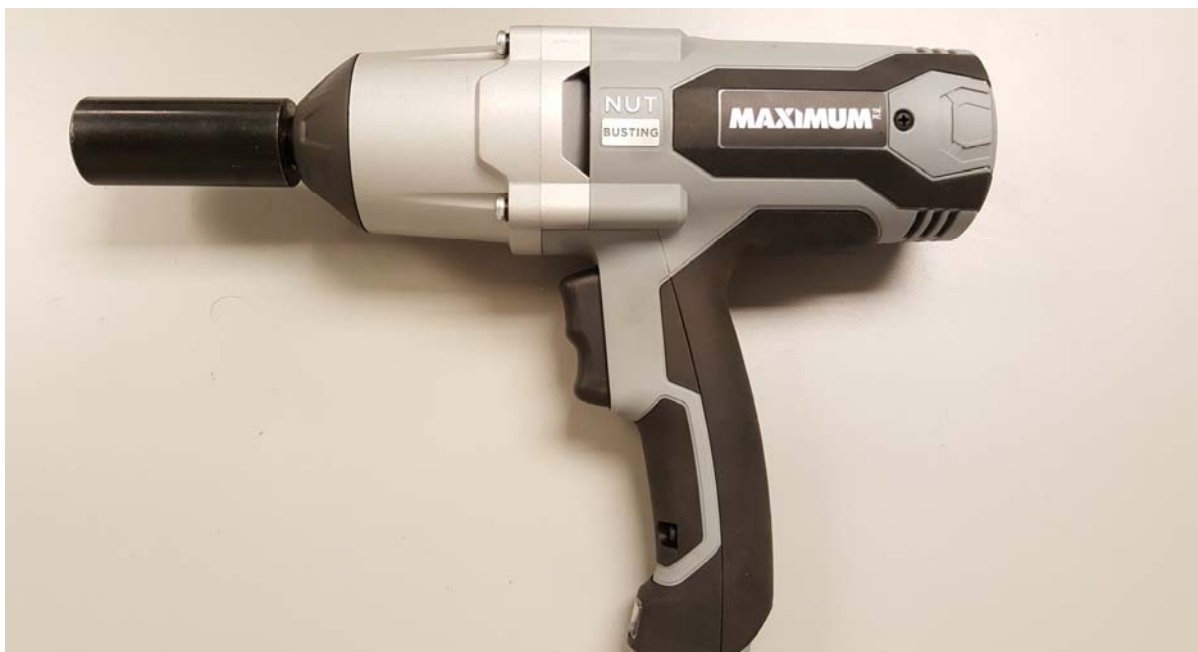
Figure 4: MAXIMUM™ ½-inch impact wrench used to adjust bolts on custom steel apparatus.
