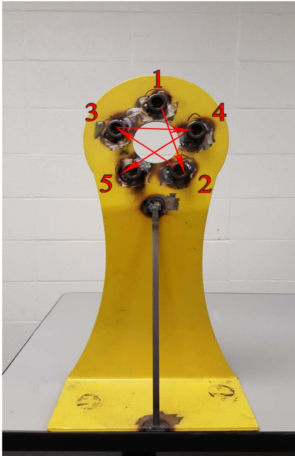
Figure 7: Experimental procedure, participants would tighten bolts in the order indicated, followed by loosening the bolts in the reverse order.
