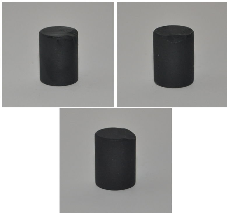
Figure 4.3: Pseudo Test Pellets with “End Square” Defects: Pellet 1 (Upper Left), Pellet 2 (Upper Right), Pellet 3 (Bottom)
