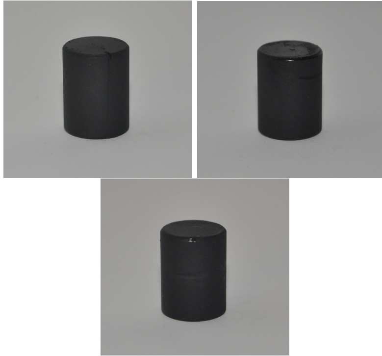
Figure 4.2: Pseudo Test Pellets with “Crack” Defects: Pellet 1 (Upper Left), Pellet 2 (Upper Right), Pellet 3 (Bottom)
