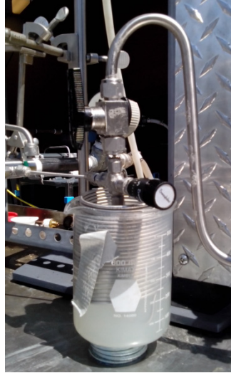
Figure 3.17: Immersed cooling coil setup connected to the ejector system.
