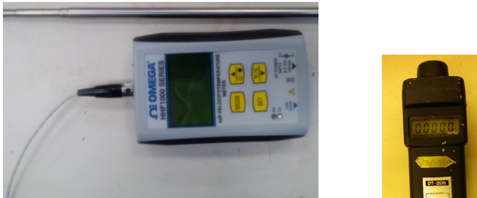
Figure 4.7: Hot wire anemometer used for air velocity measurement (left) and hand-held digital tachometer for angular speed measurement (right).
