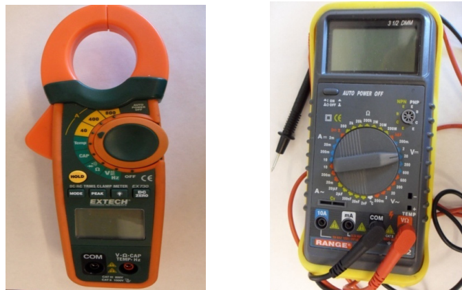
Figure 4.8: Clamp-on ammeter (left) and multi-meter (right) used for current and voltage measurement (respectively).
