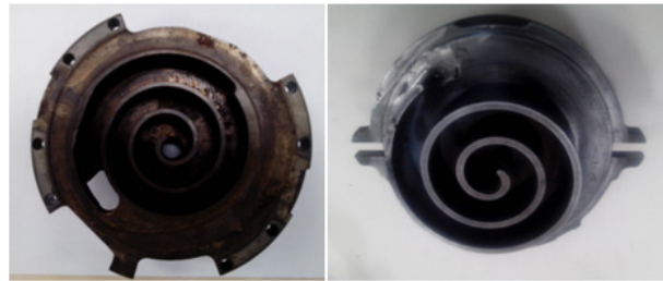
Figure 3.11: Scroll wraps of the scroll unit (fixed scroll – left side, orbiting scroll – right side).
