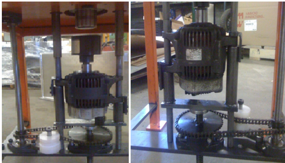
Figure 3.14: Expander-generator clutch arrangement.
