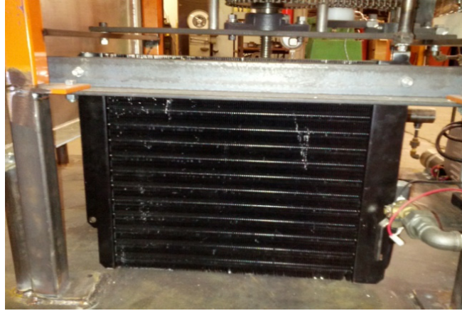
Figure 3.7: Detail photograph of the air-cooled oil cooler.
