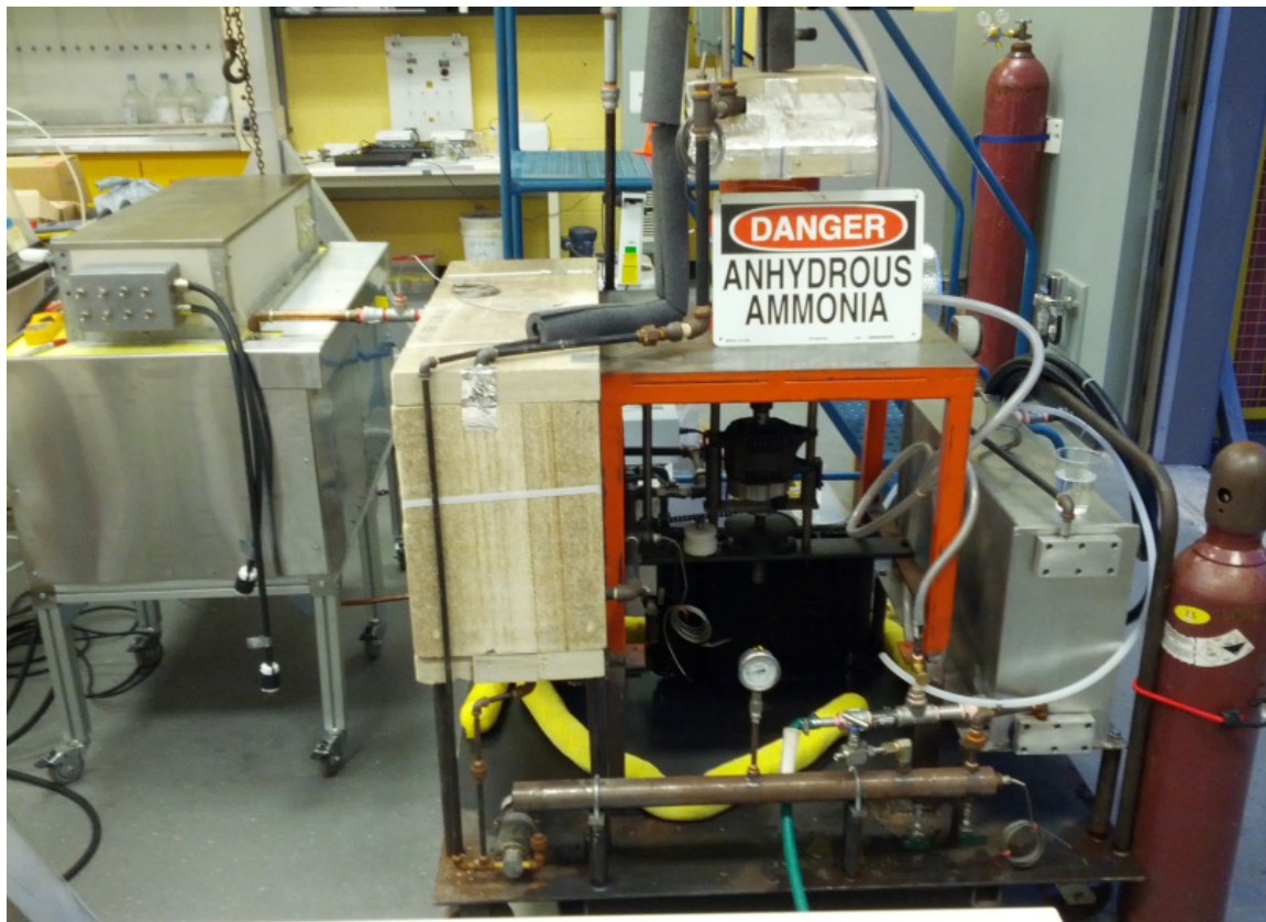
Figure 3.5: Photograph of the trigeneration system.
