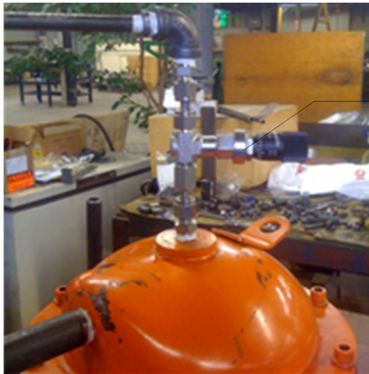
Figure 3.8: The installation of the metering valve for liquid injection.
