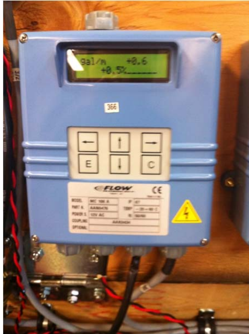
Figure 4.9: Picture of one of the five flow transceivers used in the experimentation.
