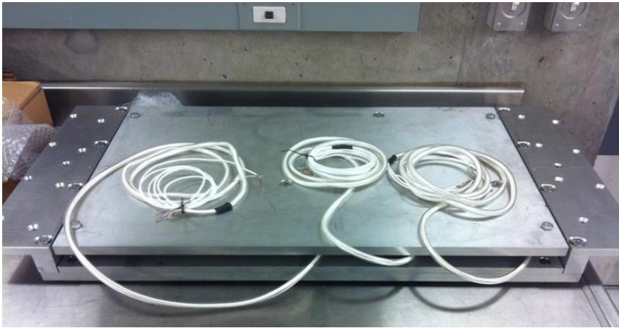
Figure 3.1: The box used to encase the load cells for aerodynamic testing
