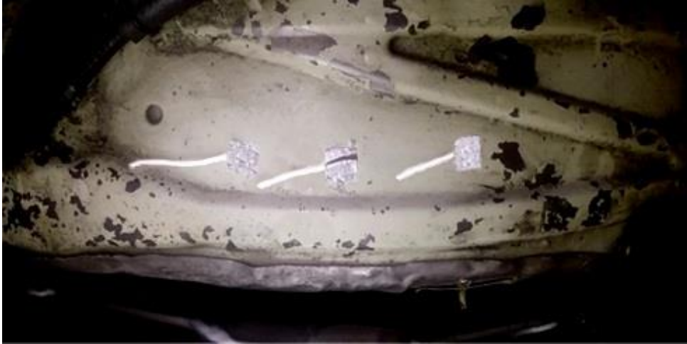
Figure 4.20: Tufts on the underbody of 944 Case 1 at 160 km/hr and 0° yaw
