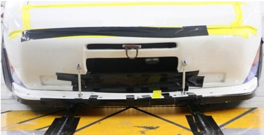
Figure II.4: 944 Case 1 with a full width front splitter, a lower radiator cover, and tape covering the hood slots
