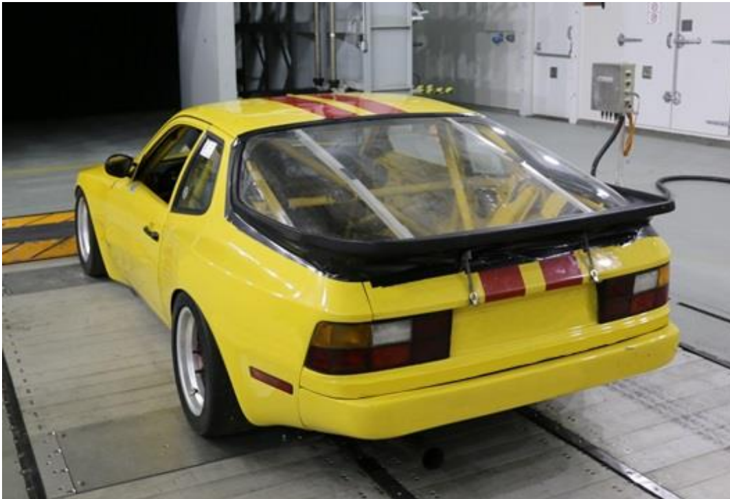
Figure II.6: 944 Case 2 showing the built-in rear wing extending out from the rear hatch
