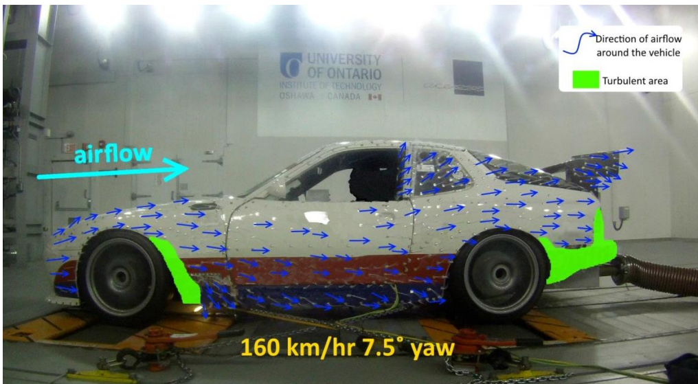
Figure 4.25: Flow visualization of the left side of 944 Case 1 in 160 km/hr wind and 7.5° yaw. Green regions indicate turbulent areas.
