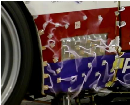
Figure 4.21: Tufts on the downwind of the front left tire of 944 Case 1 at 160 km/hr and 0° yaw.
