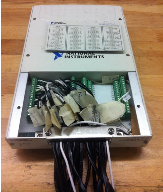
Figure 3.3: The data acquisition system (DAQ) that was used during the test
