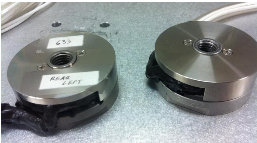
Figure 3.2: The TR3D-A-1K load cells used in the construction of the FMS box
