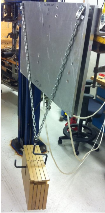
Figure IV.2: Loads suspended from the FMS box to obtain measurements on the x -axis
