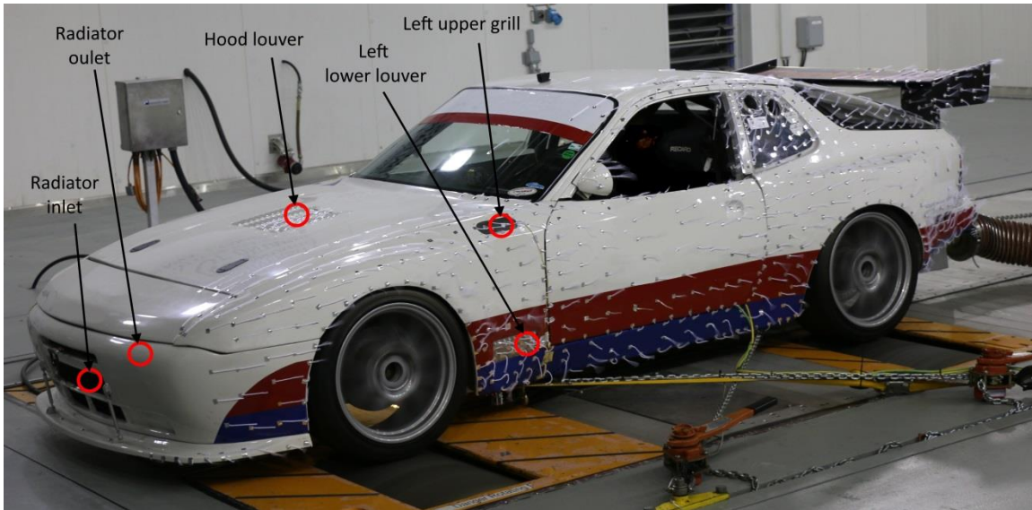
Figure 4.32: Thermocouple locations on 944 Case 1 (left side)
