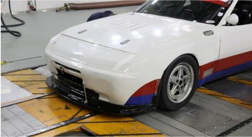
Figure II.5: 944 Case 1 with modified full width front splitter extension
