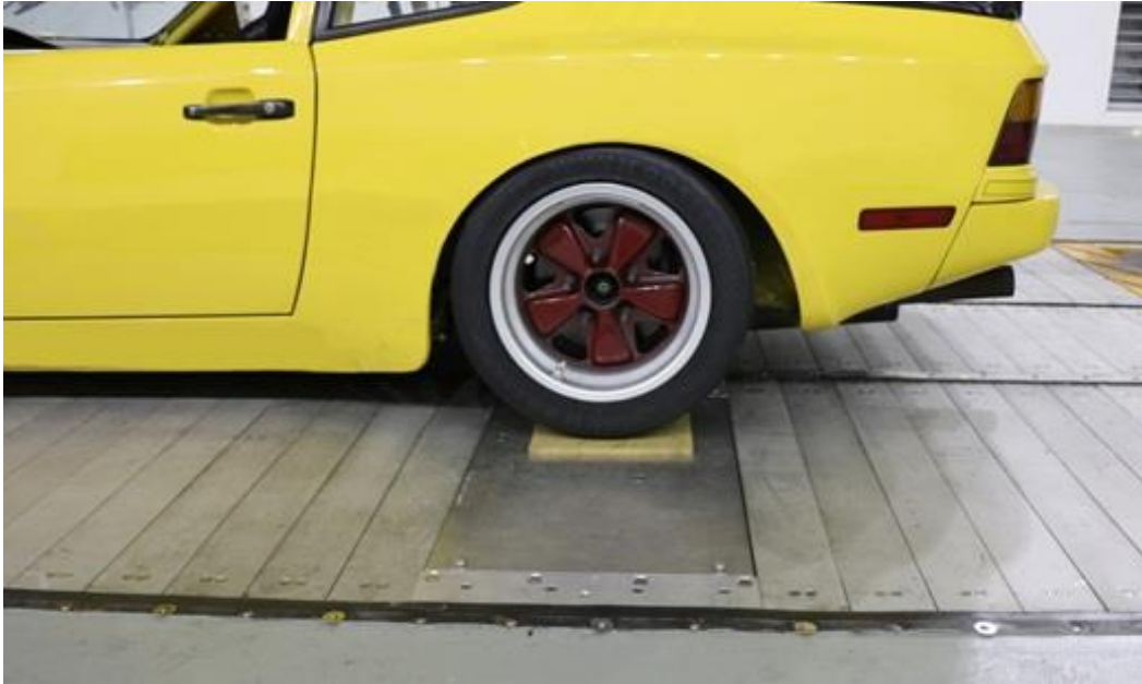
Figure II.7: A 1.5 cm rear wedge on 944 Case 2
