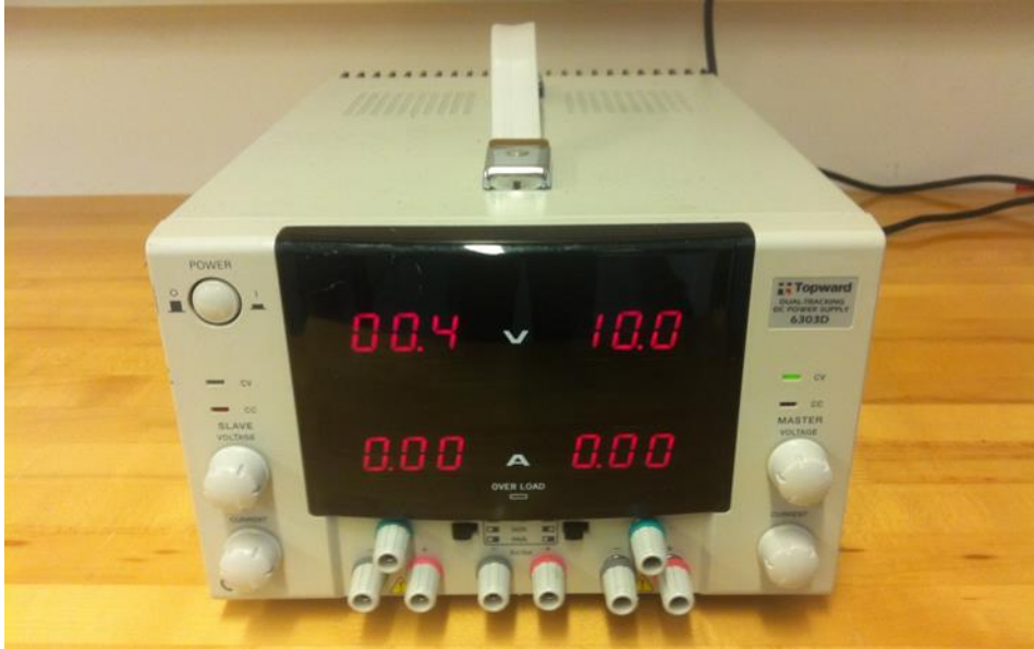
Figure 3.4: The voltage excitation source that was used to power the data acquisition system (DAQ)
