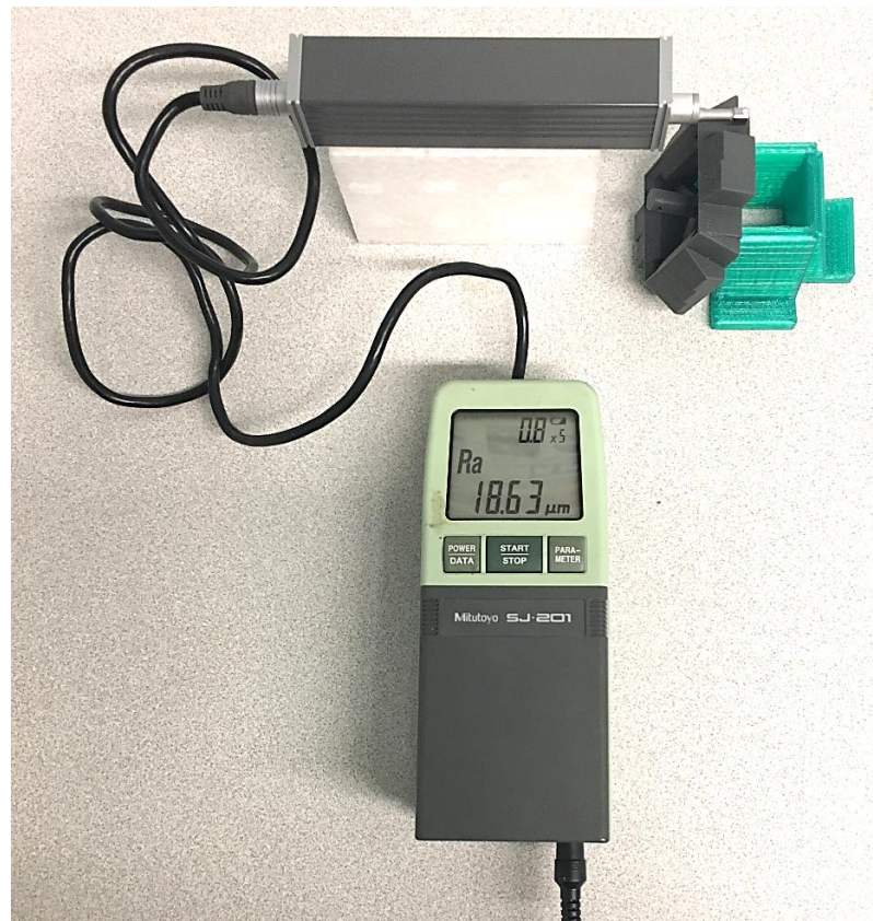
Figure 3-5 The mechanical roughness device functioning on a sample at 85^\circ .
