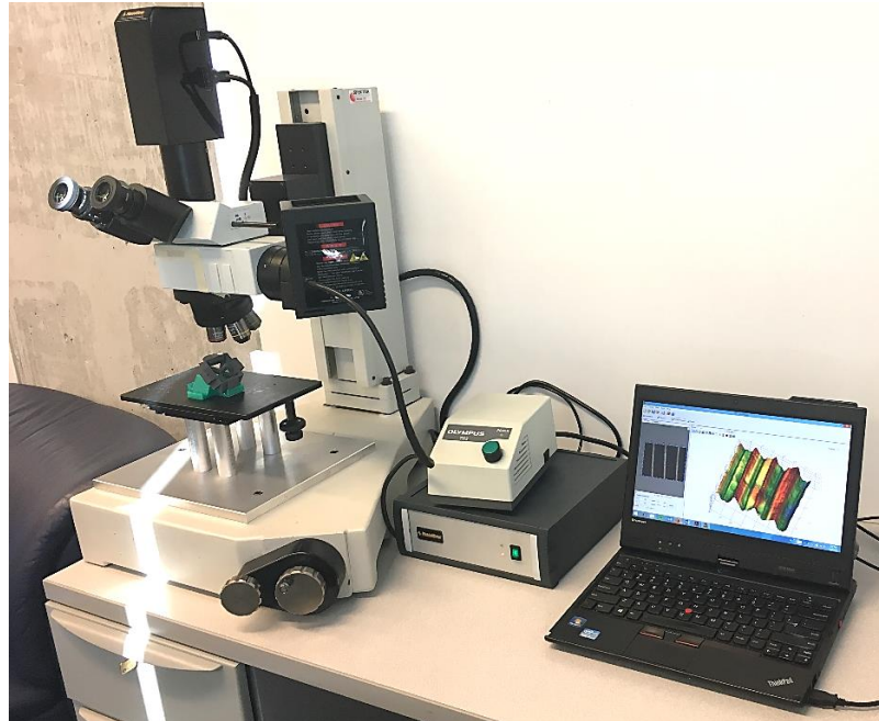
Figure 3-6 The 3D optical surface topography microscope measuring a 60° with 0.010 inch layer thickness surface.
