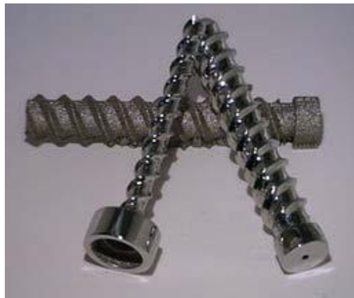
Figure 2-20 the difference between the raw surface and CNC finished part [60].
