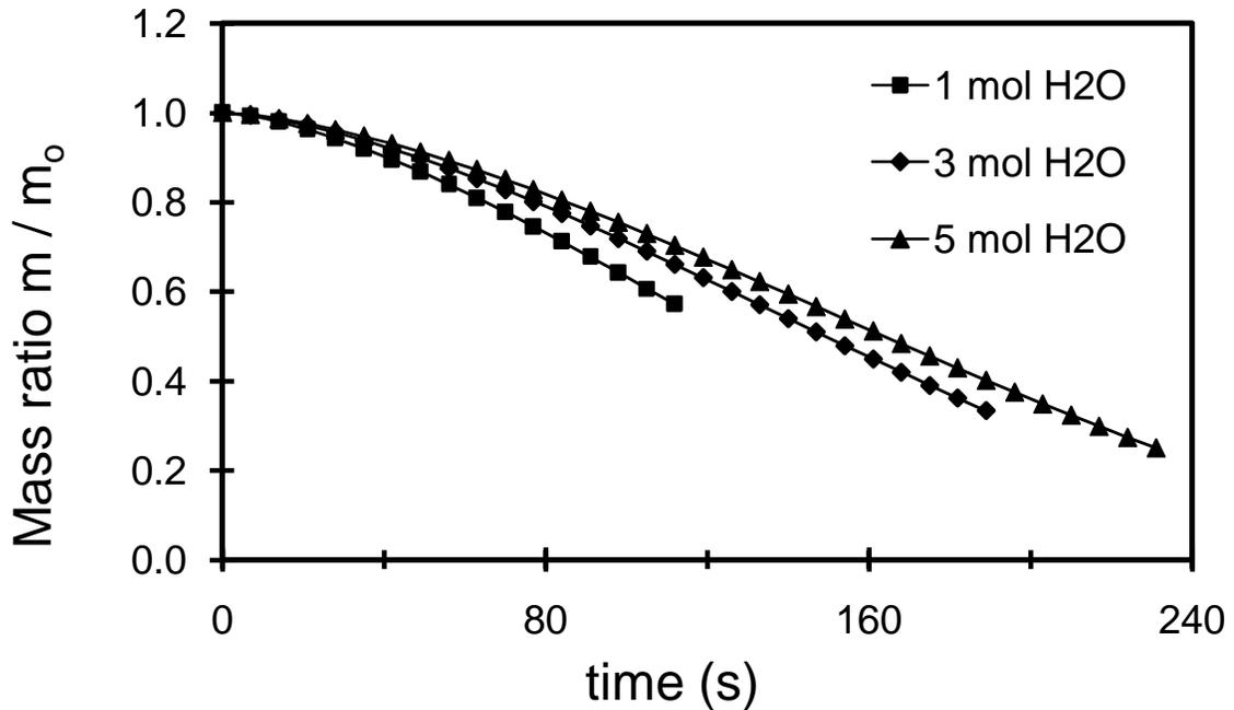
Figure 13. Mass Ratio Evolution Vs. Time with Air at 75°C, RH = 50%, HR = 0.14 kg/kg,
