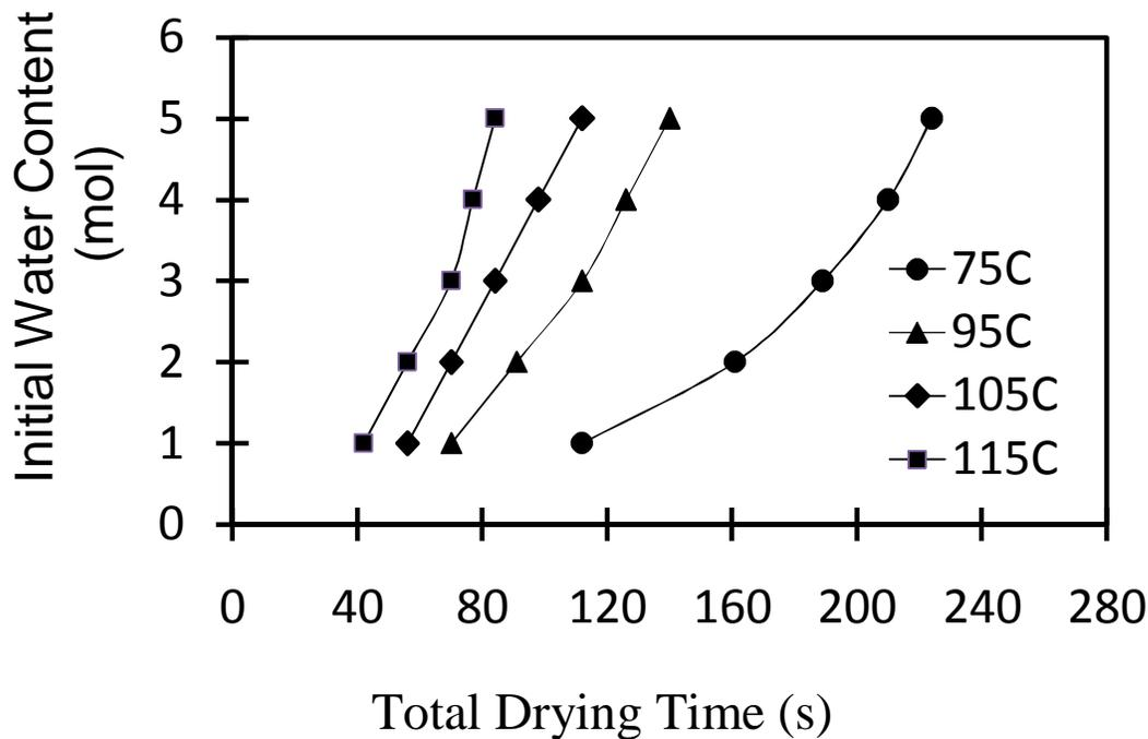
Figure 18. Initial Water Content Vs. Total Drying Time with Air Temperatures of 75°C, 95°C, 105°C and 115°C
