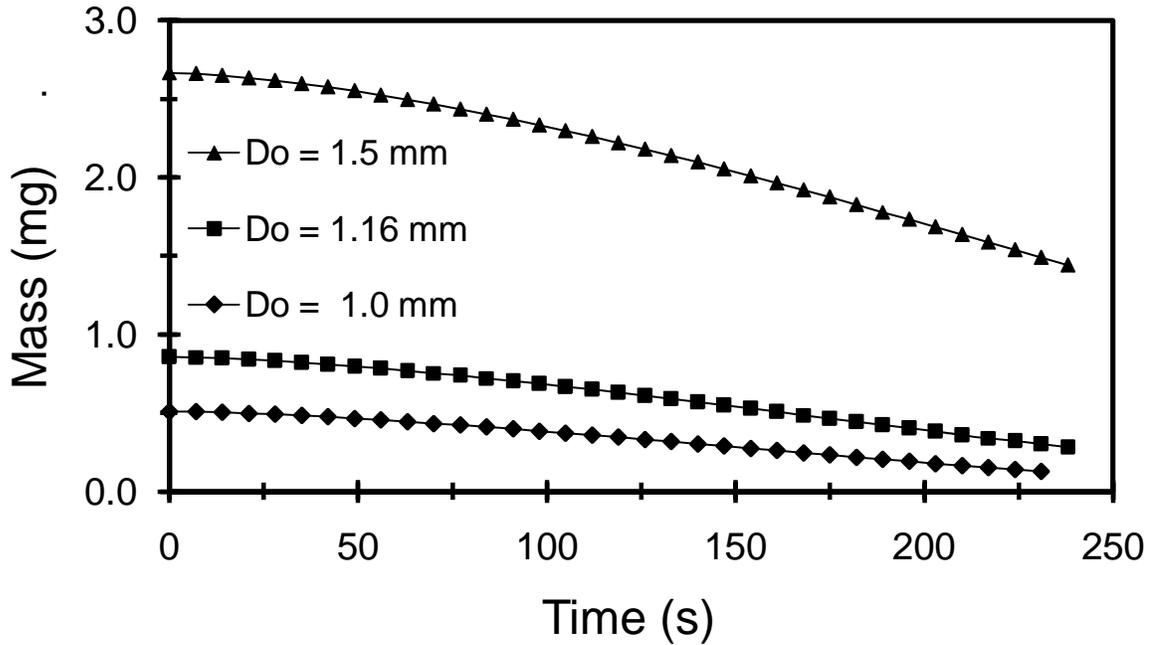
Figure 11. Change in Droplet Mass Vs. Time with Air at  $75^{\circ}\text{C}$ ,  $\text{RH} = 50\%$ ,  $\text{HR} = 0.14$ ,  $T_{\text{dp}} = 59^{\circ}\text{C}$ ,  $V = 1.75 \text{ m/s}$
