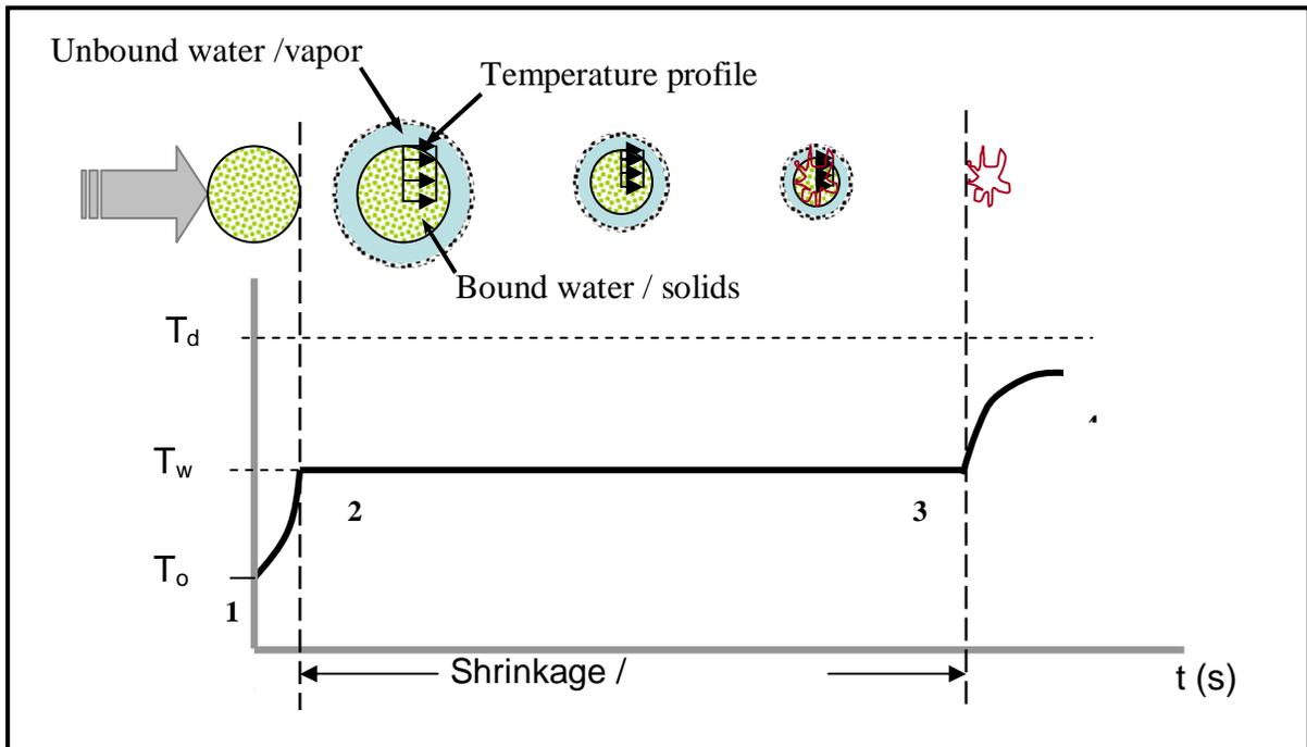
Figure 6. Stages of a Spray Drying Process
