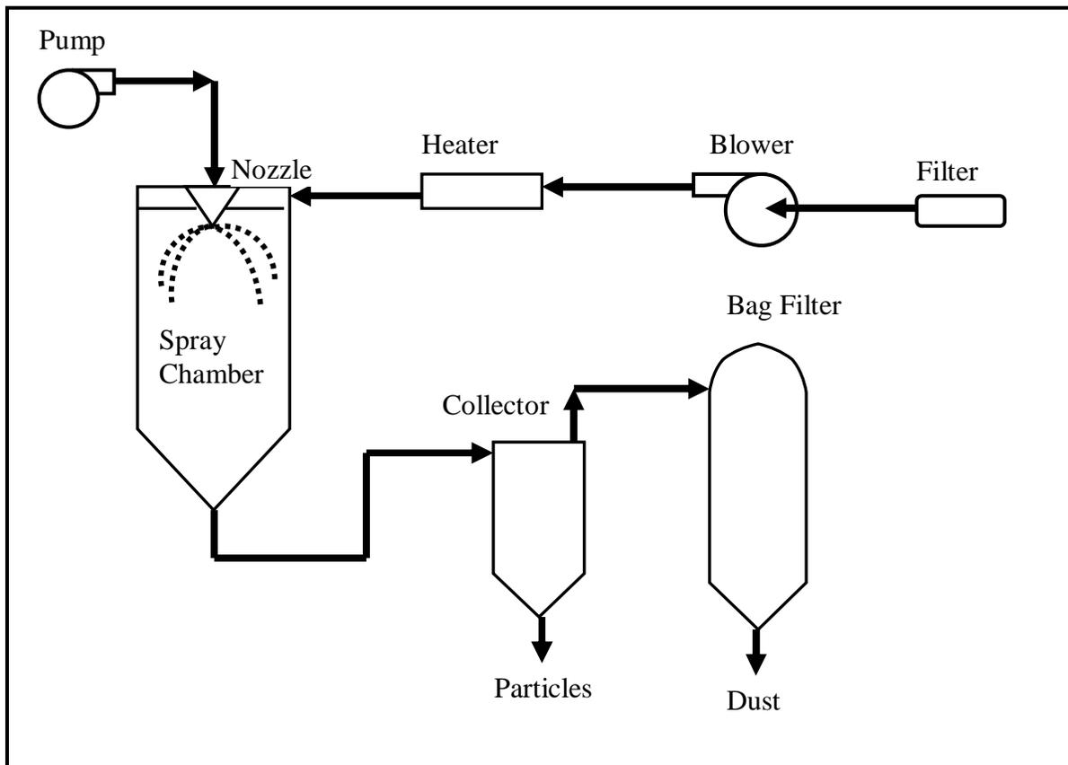
Figure 4. Schematic of a Co-Current Spray Dryer System
