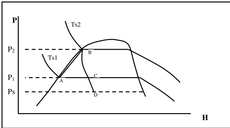
Figure 2. Pressure-Enthalpy Diagram of Flashing Process –ABCD–
