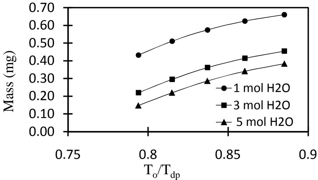
Figure 17. Droplet Mass Change vs. Ratio of Initial Droplet Temperature to Changing Air Temperature at RH = 50%, Do = 1 mm, V = 1.75
