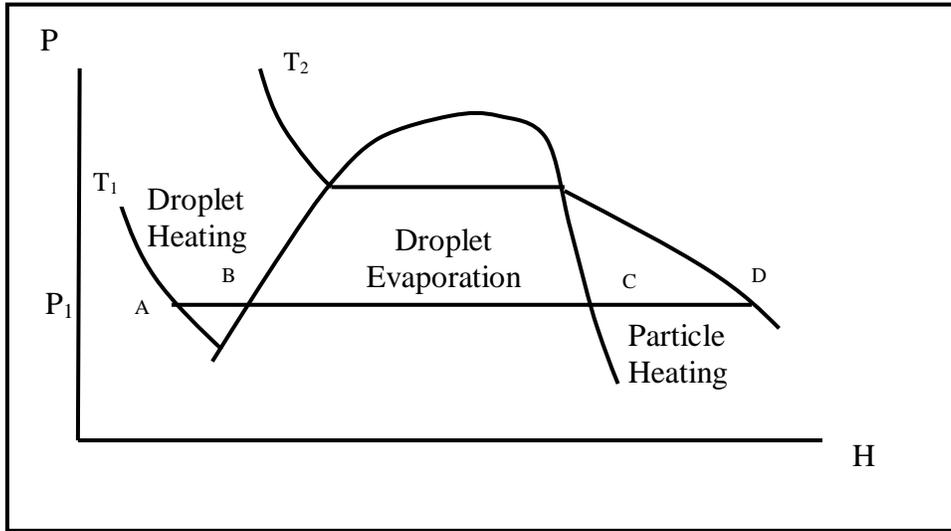
Figure 5. Phase Diagram of a Spraying Process–ABCD–
