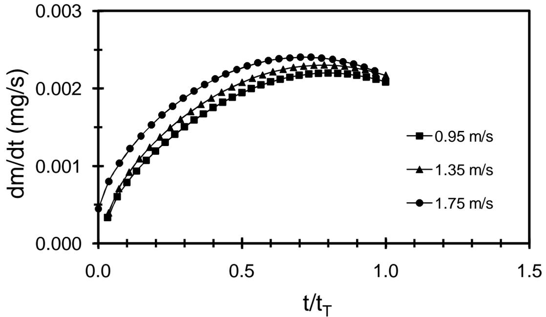
Figure 12. Effects of Air Velocity on the Evaporation Rate with Air at 75°C, RH = 50%, 3 mol H<sub>2</sub>O, T<sub>dp</sub> = 59°C, HR = 0.14 kg/kg, D<sub>o</sub> = 1.0 mm
