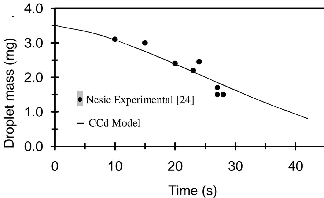
Figure 8. Experimental (Nestic [24]) vs. Predicted (CCd) Drying History of Colloidal Silica in Air at  $178^\circ\text{C}$
