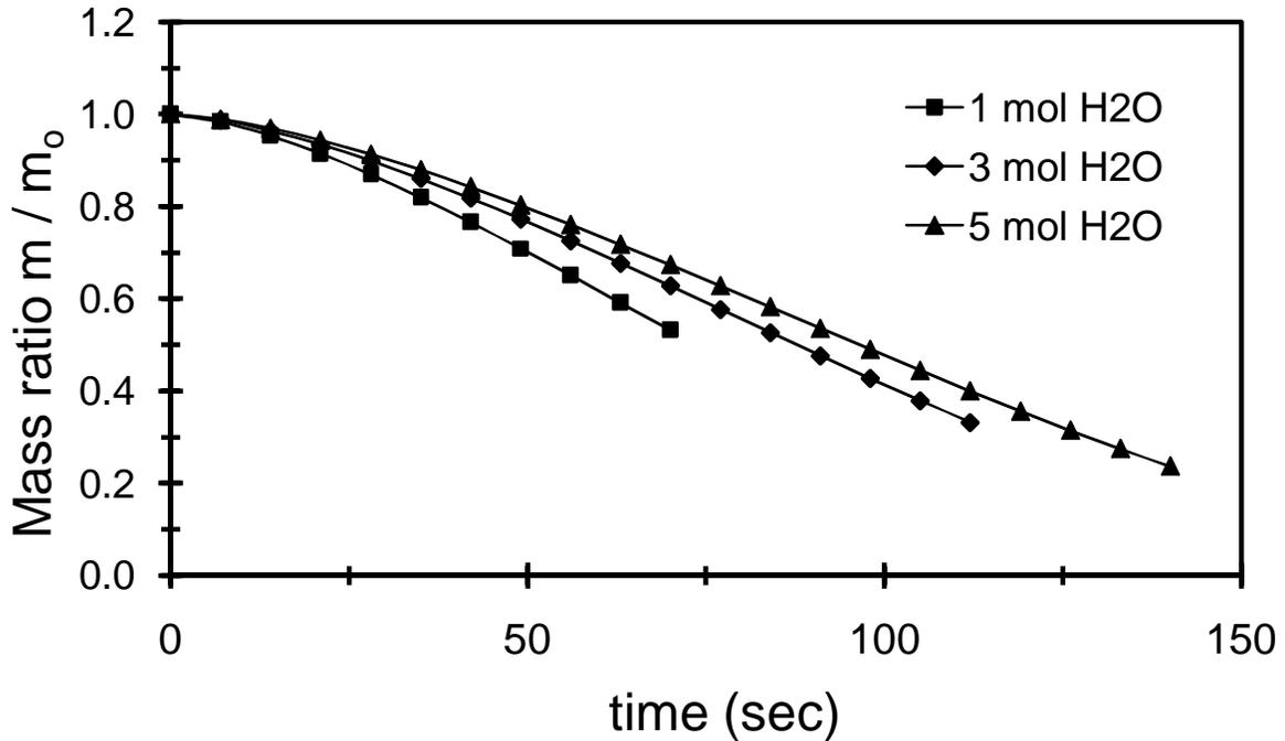
Figure 14. Mass Ratio Evolution with Air at 95°C, RH = 50%, HR = 0.14 kg/kg, T<sub>dp</sub> = 77°C, D<sub>o</sub> = 1.0 mm, V = 1.75 m/s
