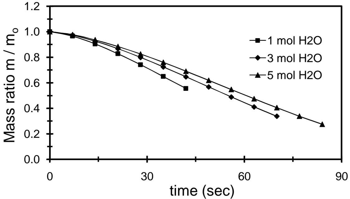
Figure 16. Mass Ratio Evolution Vs. Time with Air at 115°C, RH = 50%, HR = 0.14 kg/kg, T<sub>dp</sub> = 95°C, D<sub>o</sub> = 1.0 mm, V = 1.75 m/s
