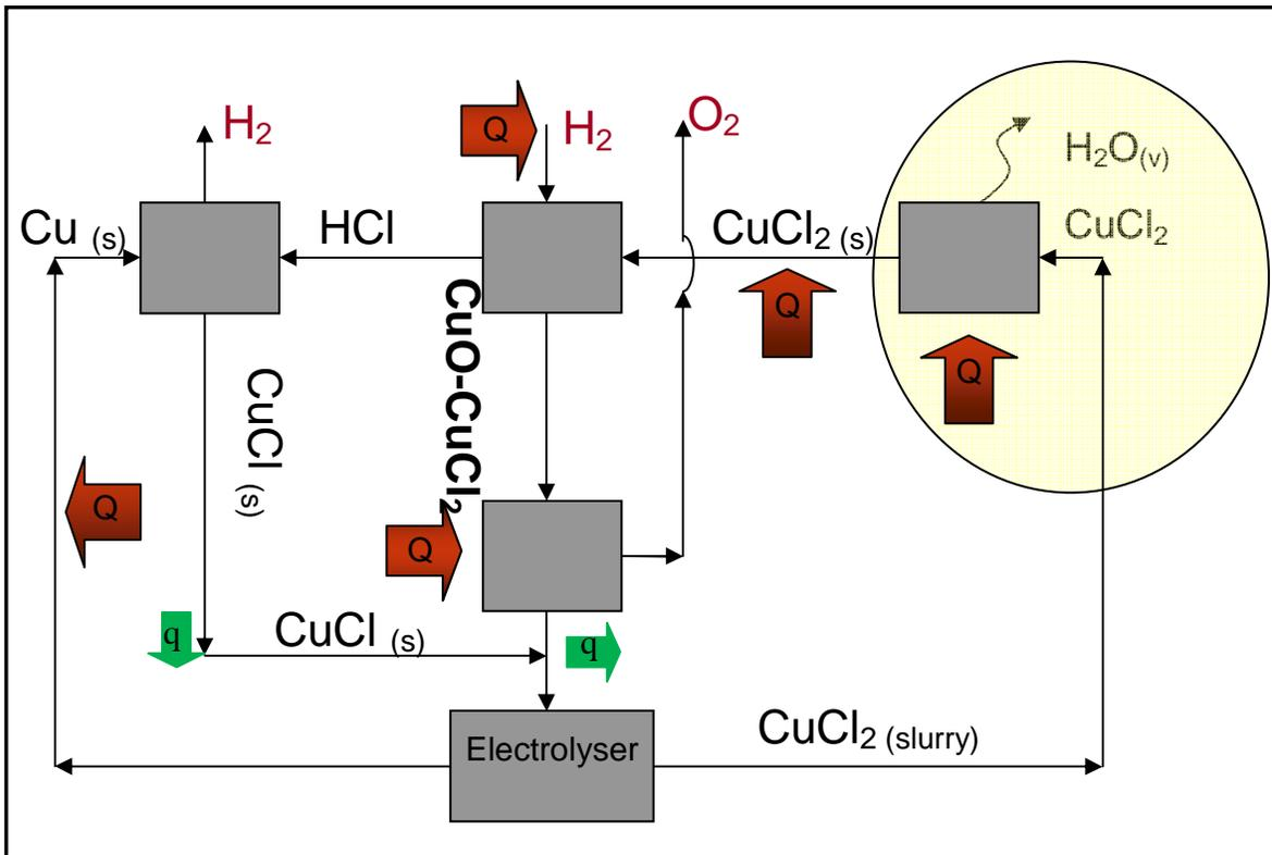
Figure 1. Simplified Schematic of a Thermo-Chemical Copper-Chlorine Cycle
