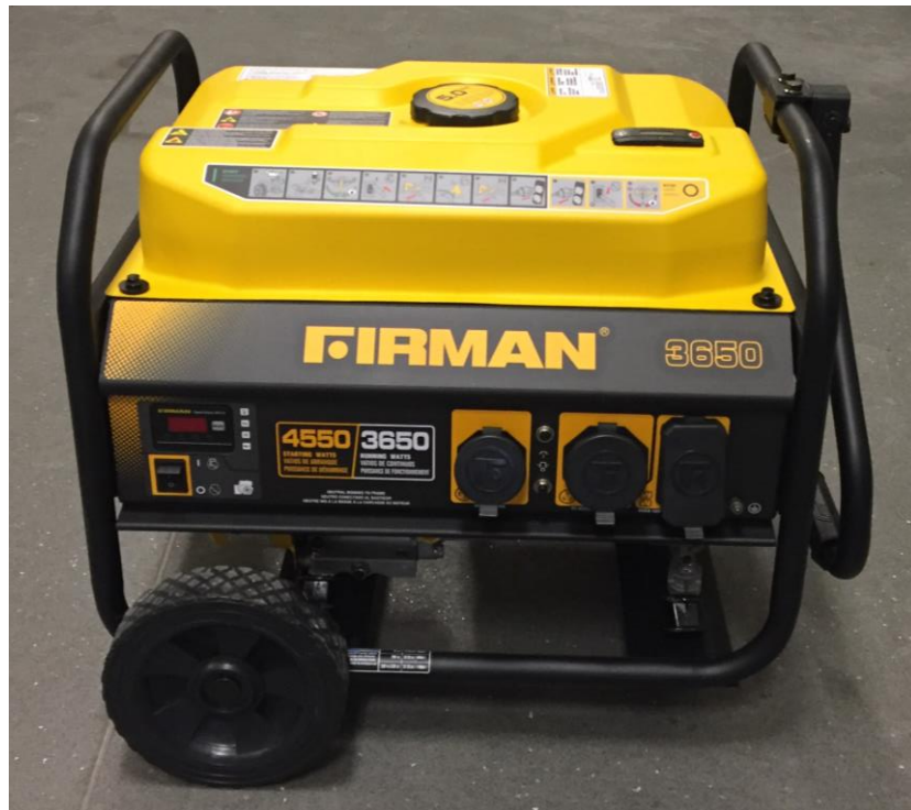
Figure 3.1: FIRMAN P03602 portable gasoline generator used in the experiments
