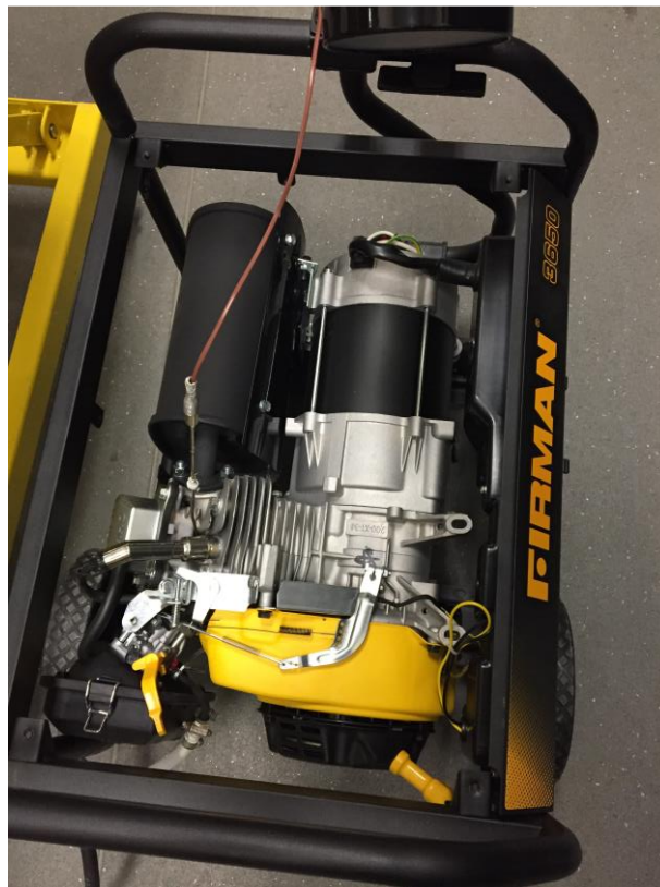
Figure 3.2: Spark ignition engine of FIRMAN P03602 portable gasoline generator
