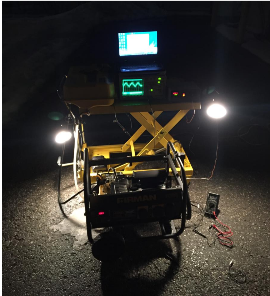
Figure 3.8: During the operation of the experimental setup operating at varying fuel blend ratios of gasoline and ammonia placed outside the CERL
