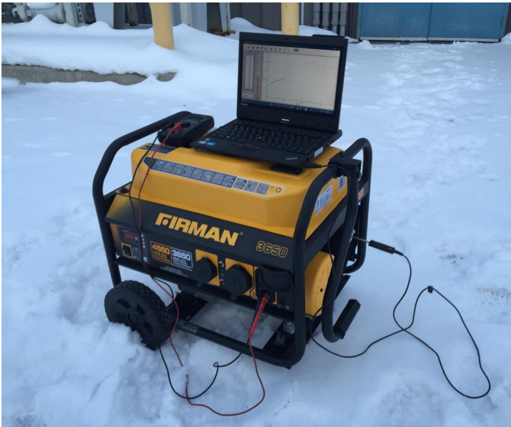
Figure 3.5: The setup without any engine modifications trailed with only gasoline at this stage of the experimental studies
