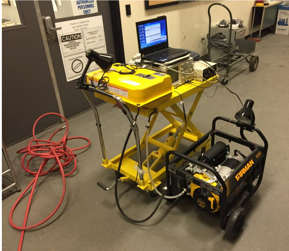
Figure 3.6: The setup after with necessary modifications to be used with different ratios of ammonia and gasoline blends at this stage of the experimental studies with the inclusion of the instruments that will be used in the measurements
