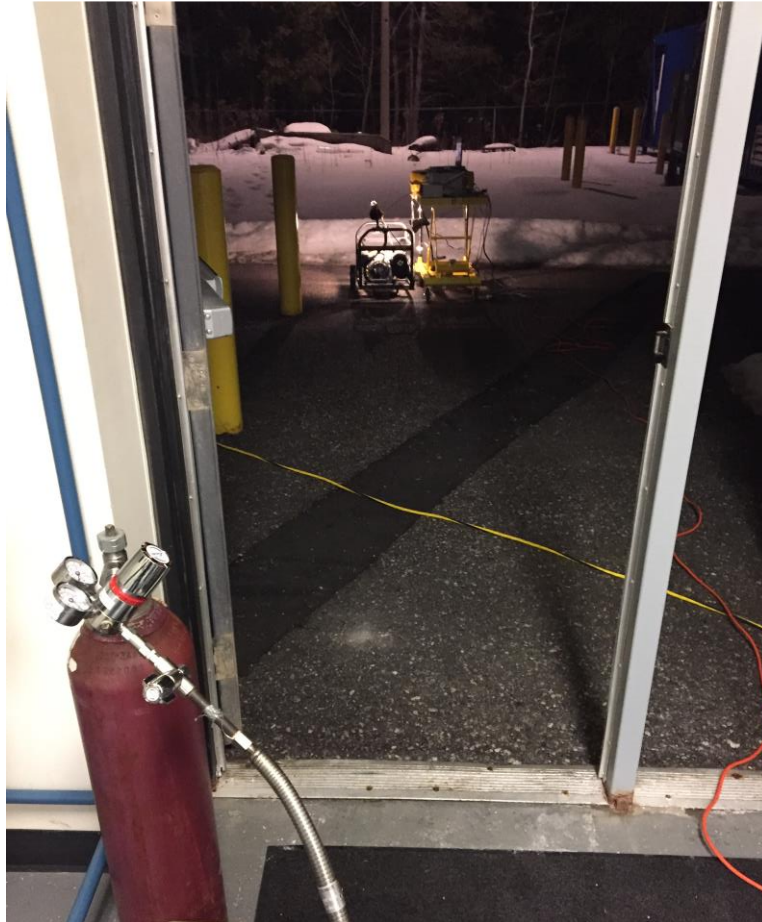
Figure 3.7: The setup placed outside CERL building with the ammonia cylinder stored inside the building and connected with the use of extra piping
