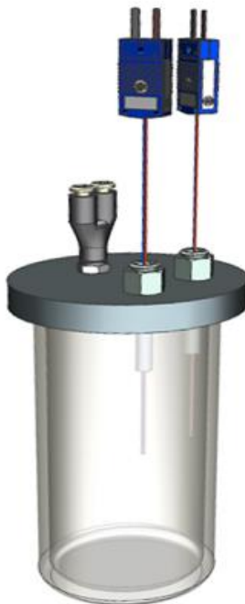
Figure 3.4 PTFE cap for melting the electrolyte and cycling nitrogen gas (inert) to purge out undesired gas.
