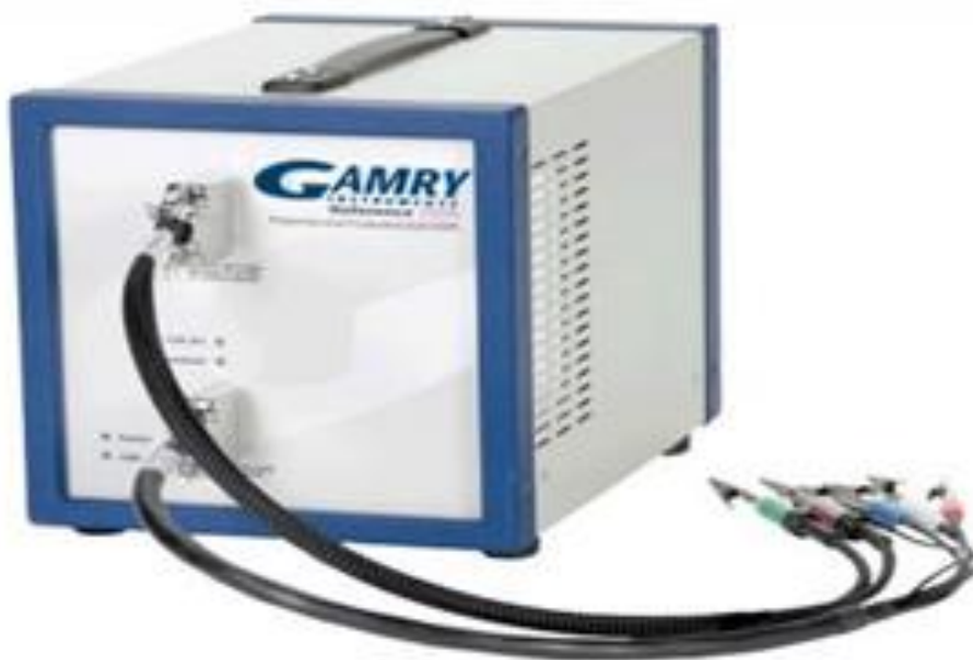
Figure 3.6 Gamry reference 3000 used in the experiment to perform electrochemistry studies.
