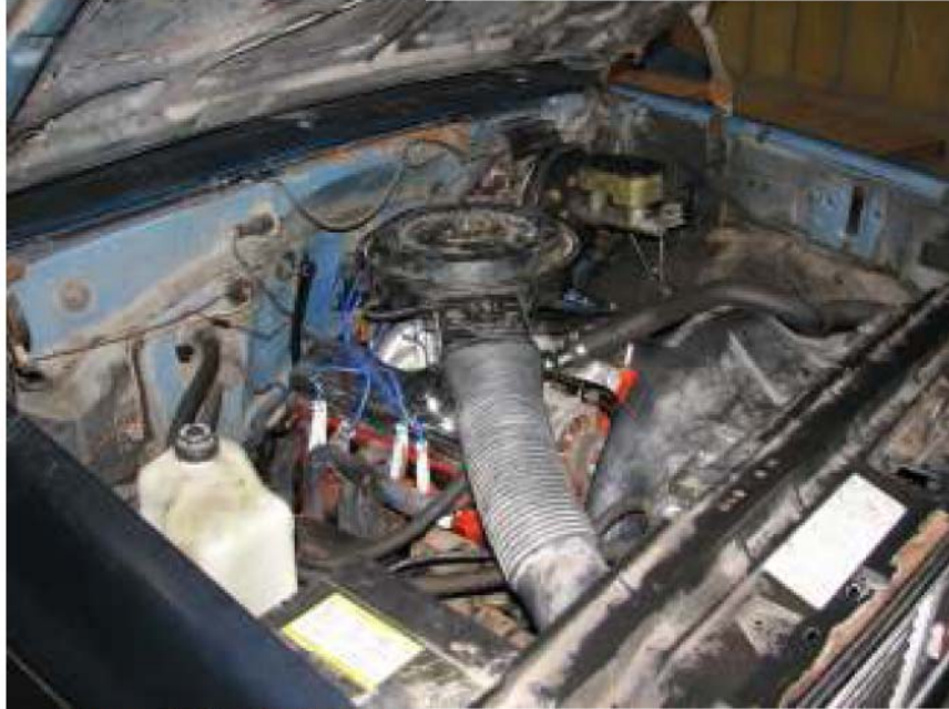
Figure 4.29: 1976 Chevrolet small block 350 CID 5.7L V8.
