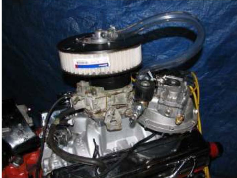
Figure 4.11: Engine on hydrogen components.
