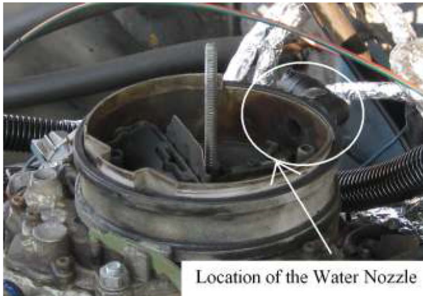
Figure 4.36: Water nozzle location on the spacer located on top of the carburetor.
