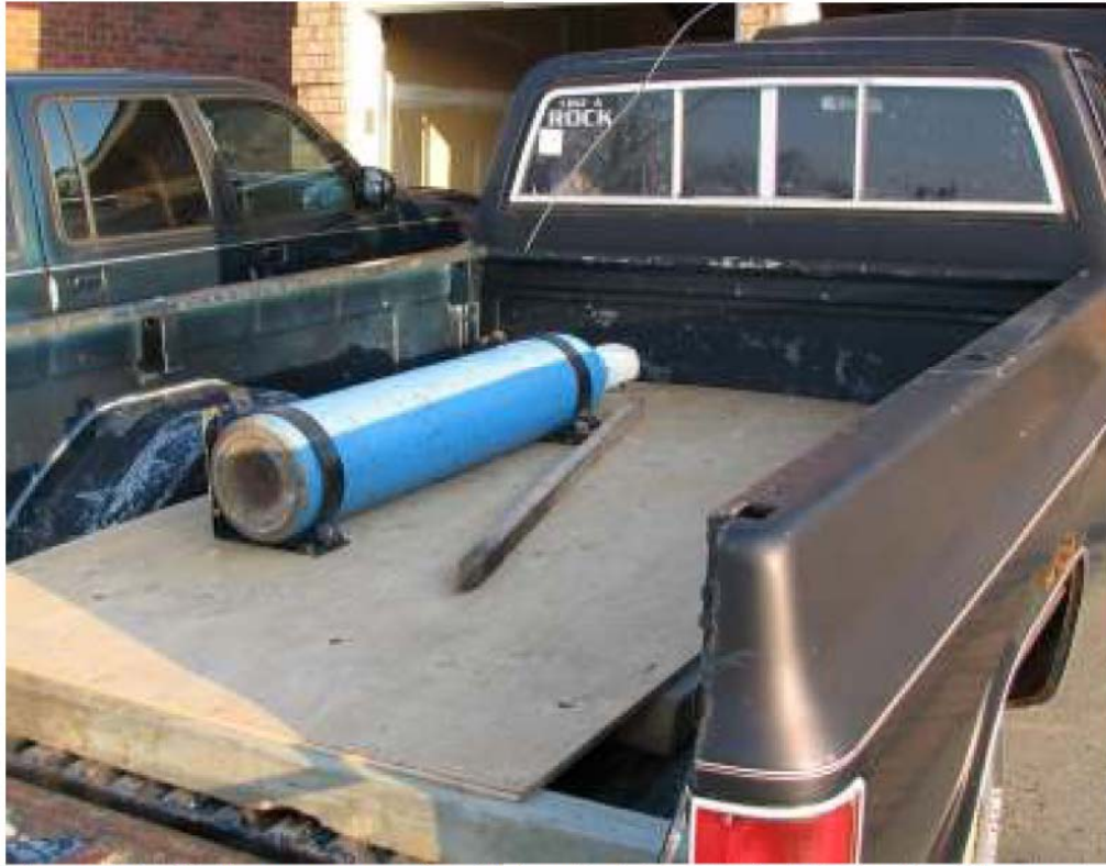
Figure 3.7: Hydrogen test tank with brackets installed at the back of the truck.
