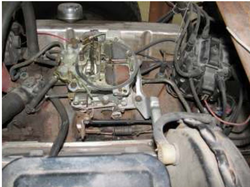
Figure 4.30: 4-barrel Rochester quadrajet M4MED carburetor.
