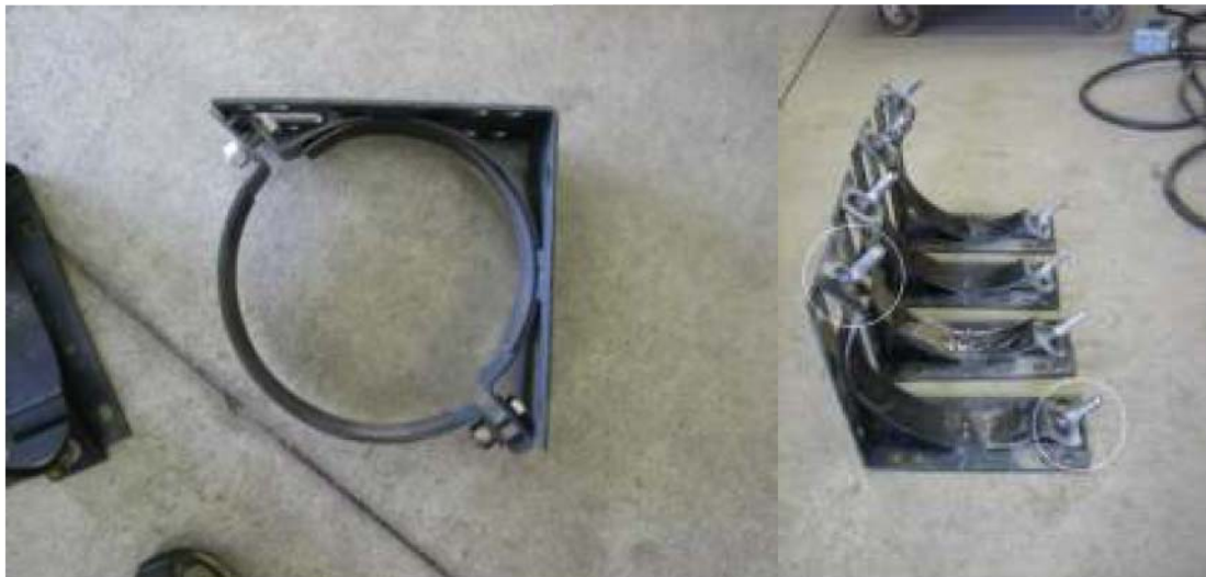
Figure 3.6: Four mount brackets with welded screws on the brackets.
