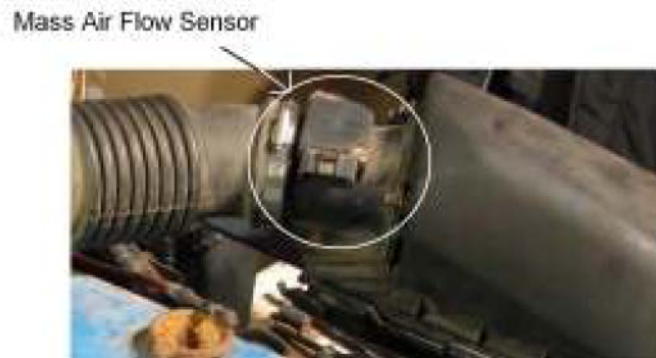
Figure 4.1: Typical location of a mass air flow sensor.
