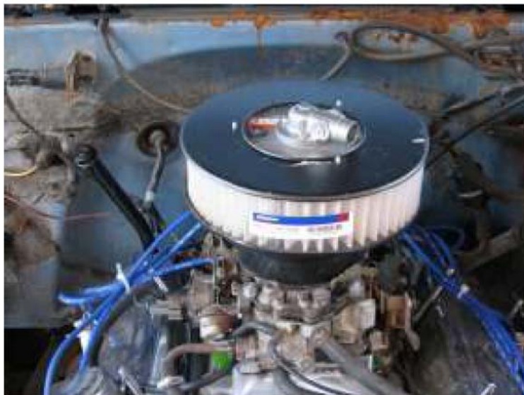
Figure 3.3: Gas mixer, air filter with cover, spacer and adapter assembly on top of the carburetor.
