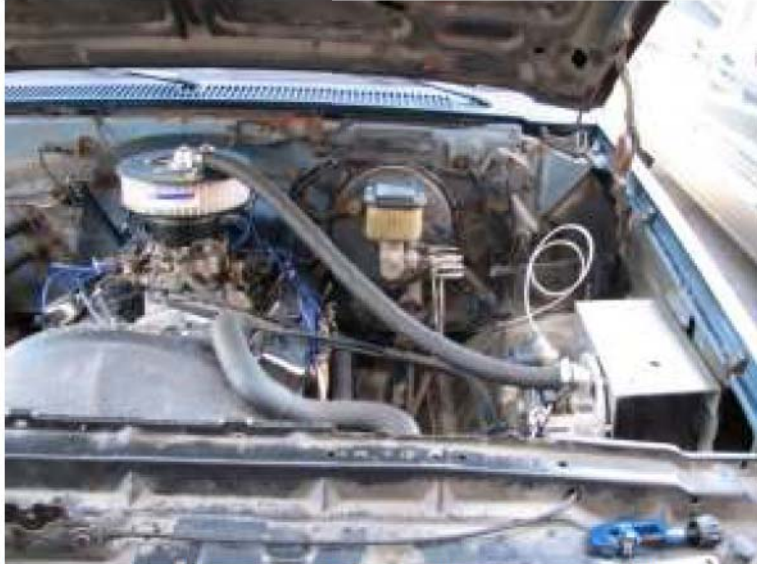
Figure 3.4: Hose connected from regulator to the mixer assembly, for hydrogen fuel.
