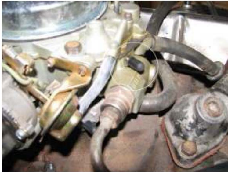
Figure 3.1: vacuum lines removed and capped on the carburetor.
