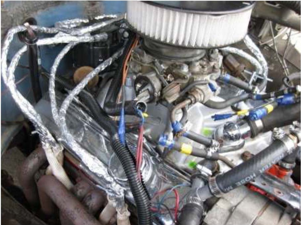
Figure 4.39: Spark plug wire ground modification for post-ignition elimination.
