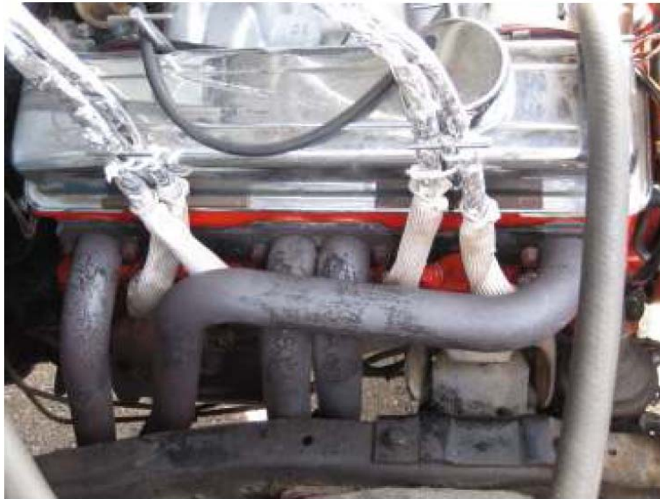
Figure 4.38: After-market headers with heat resistant covers for the spark plug wires.
