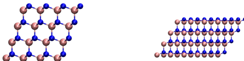
FIGURE 1.8: Left: Cubic boron nitride, view from the top. Right: Cubic boron nitride, view from the side.
