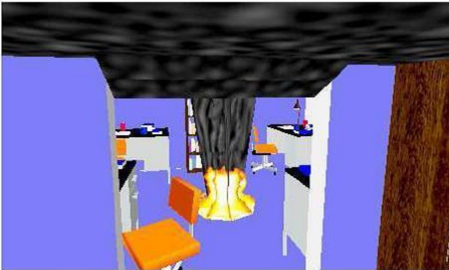
Figure 6.2: An intense pool fire in a student office; 100 seconds after ignition, the room is nearly filled with smoke. Reprinted with permission.
