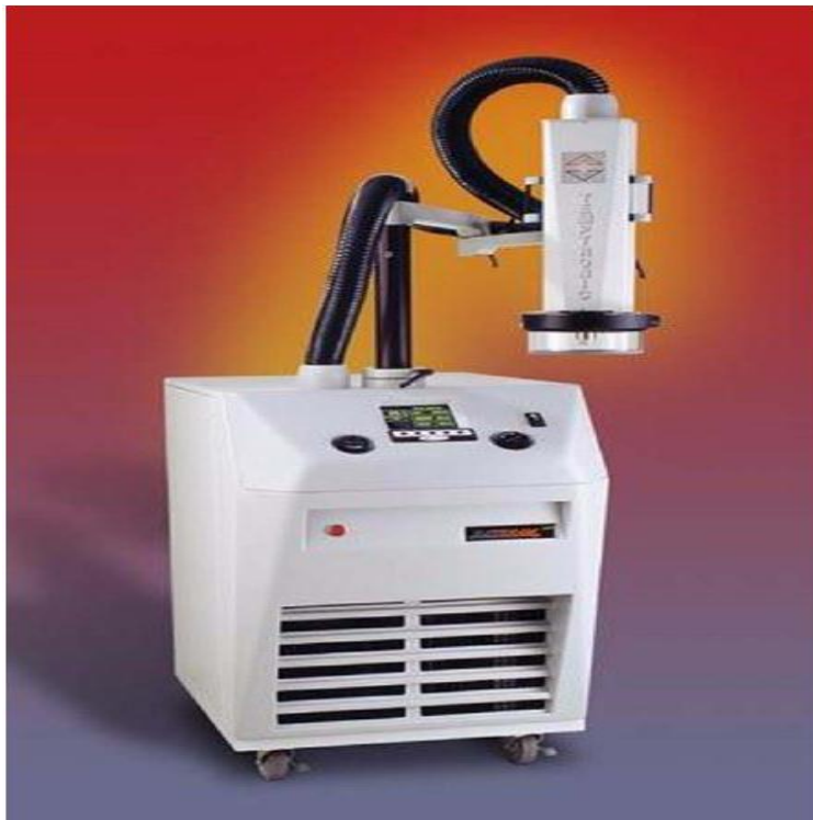
Figure 5.1 The Temptronic device to heat and cool the test chamber.
