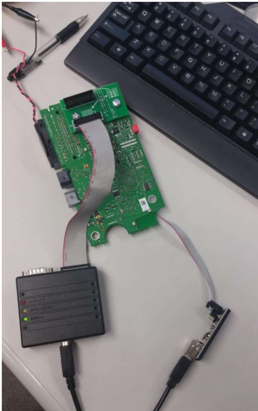
Berla iVe connectors attached to JTAG components connected to Ford SYNC module
