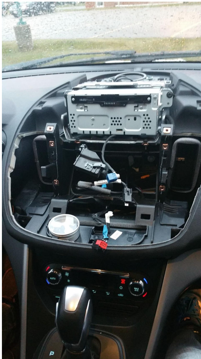
Example of Ford SYNC module retrieval process
