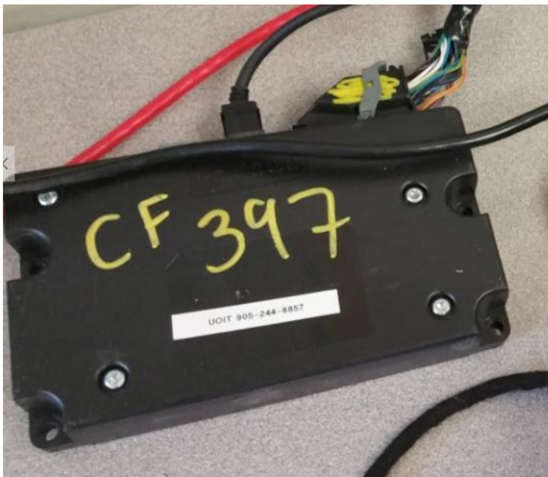
Ford SYNC storage module (JTAG acquisition done on board residing inside encasement)
