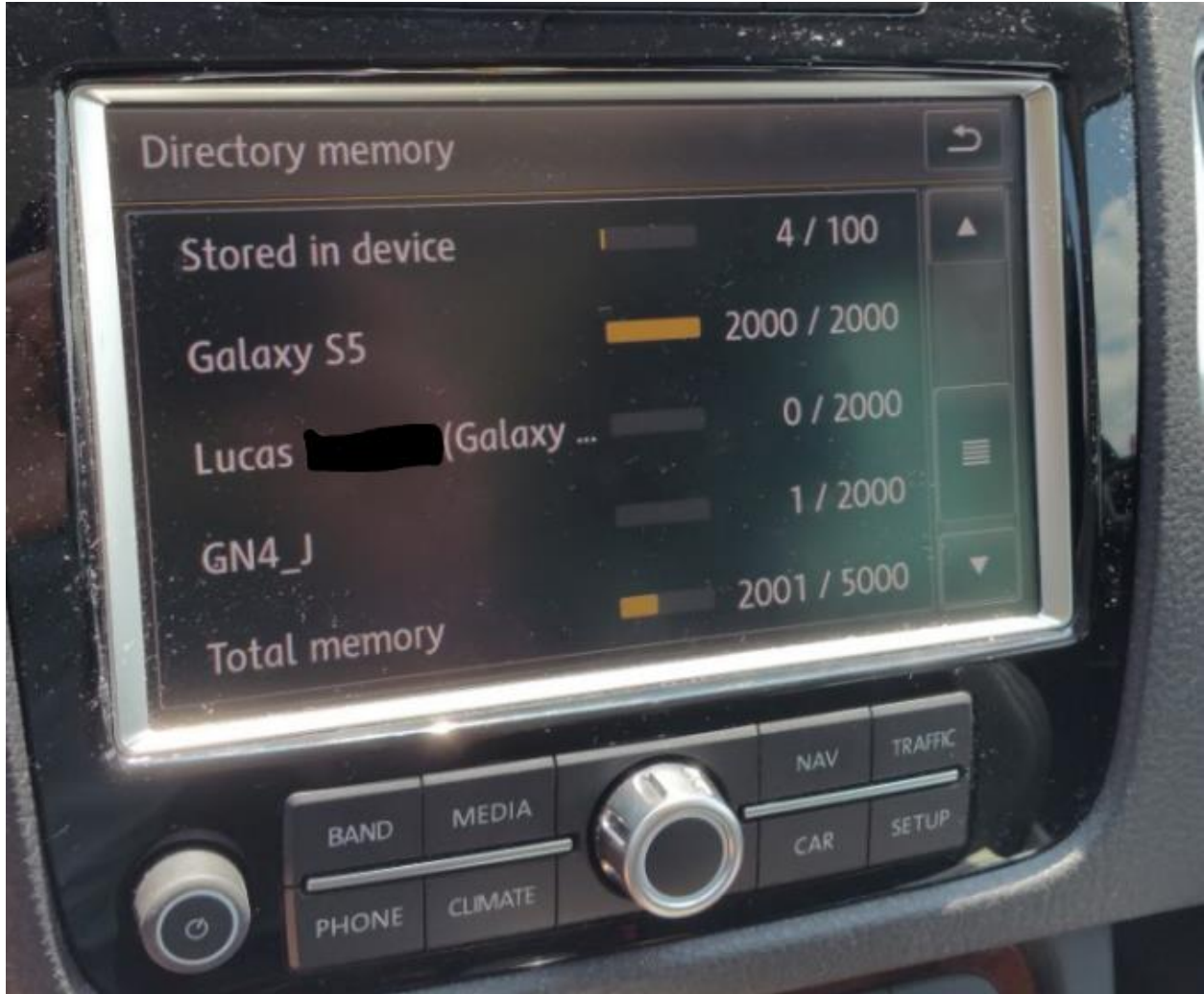
Number of items in memory per connected devices (current and prior)
